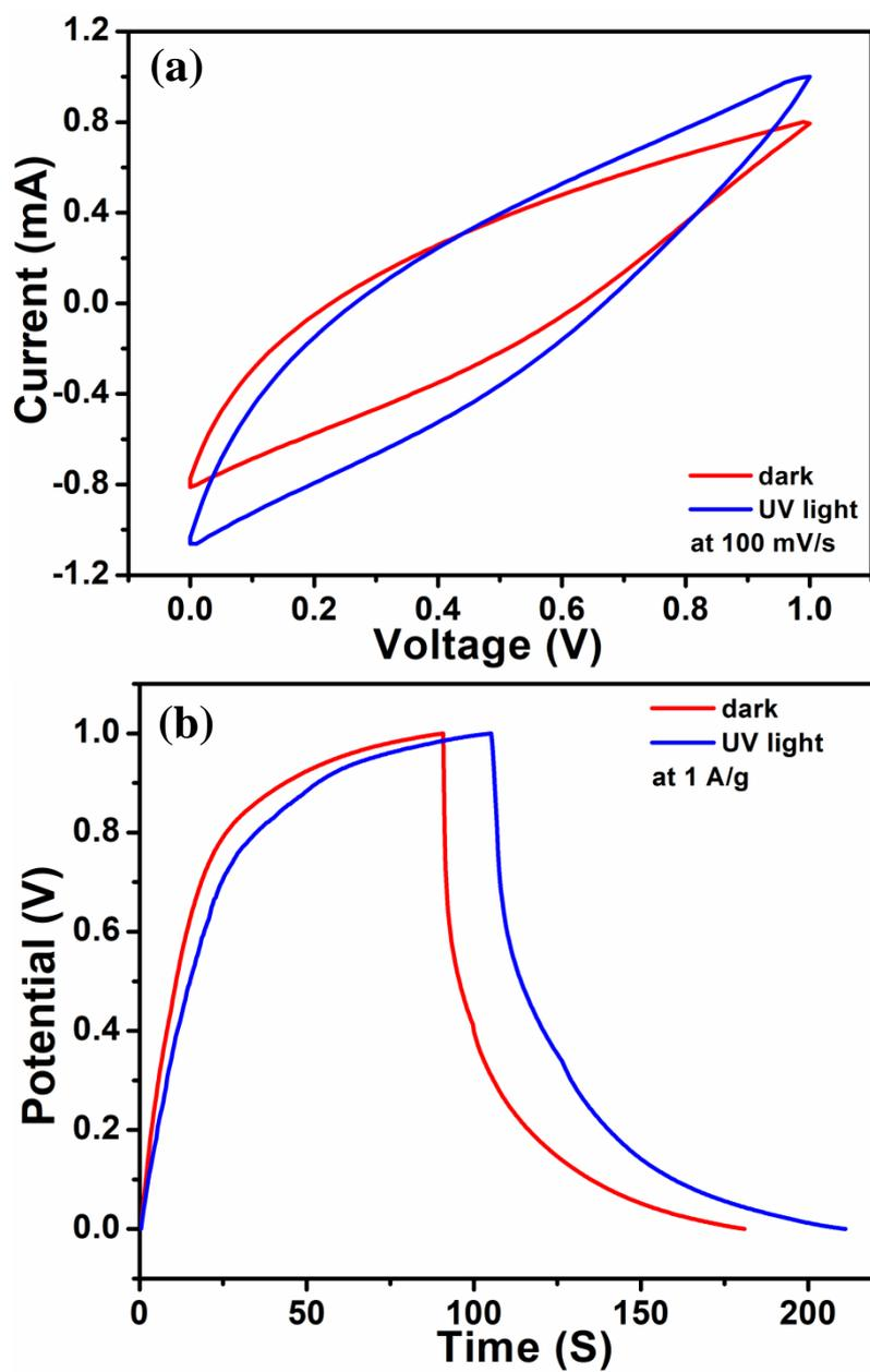
**Fig. S16.** Overlay of (a) Cyclic voltammograms at 100 mV/s scan rates and (b) GCD plots at 1 A/g current density of PTNCO-1 under dark and UV light condition at 2 electrode system.
