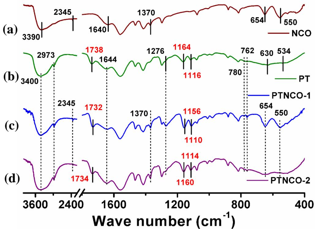
Fig. S2. FTIR spectra of (a) NCO, (b) PT, (c) PTNCO-1 and (d) PTNCO-2.
