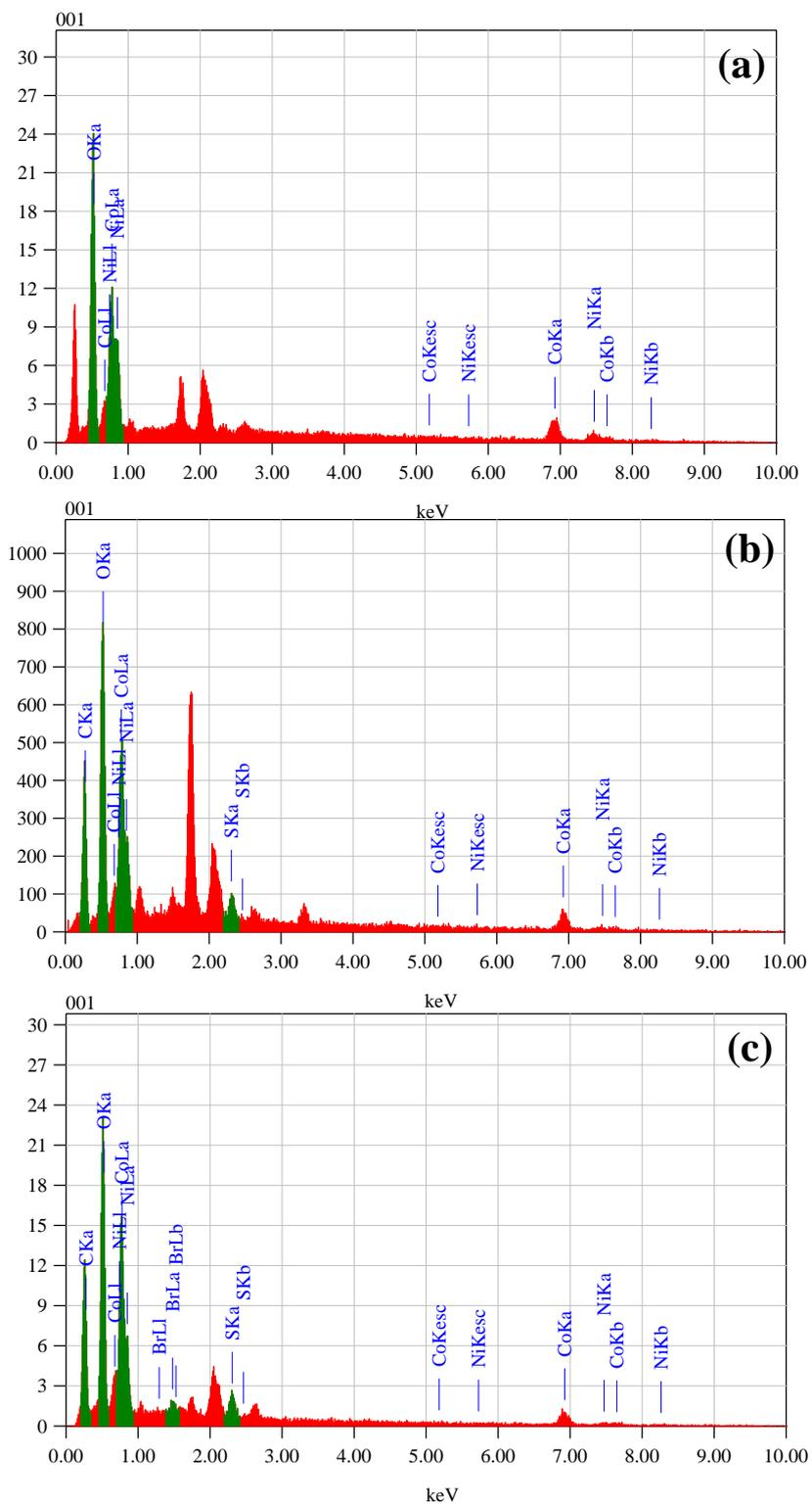
**Fig. S5.** EDX spectrum analysis of (a) NCO, (b) PTNCO-1 and (c) PTNCO-2.
