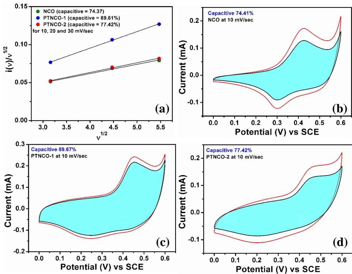
**Fig. S14.** Plot of (a)  $i(v)/v^{1/2}$  vs  $v^{1/2}$  for all three electrodes, Dunn method analysis of capacitance contribution of (b) NCO, (c) PTNCO-1 and (d) PTNCO-2 three electrodes at 10 mV/sec scan rate.
