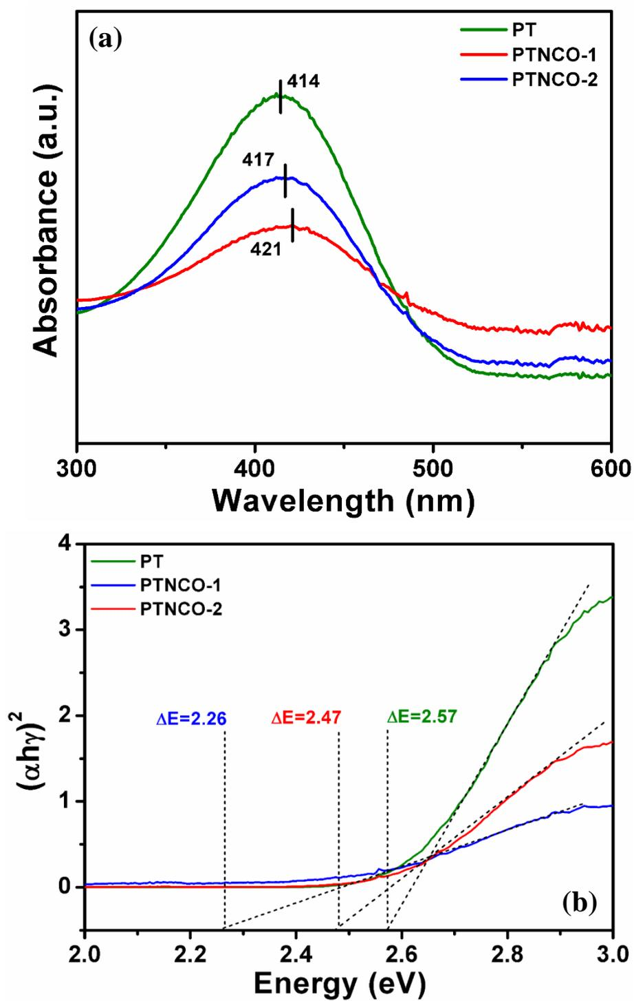
**Fig. S7.** Images of (a) UV-Vis spectra and (b) Tauc plot of PT, PTNCO-1 and PTNCO-2 in THF solution.
