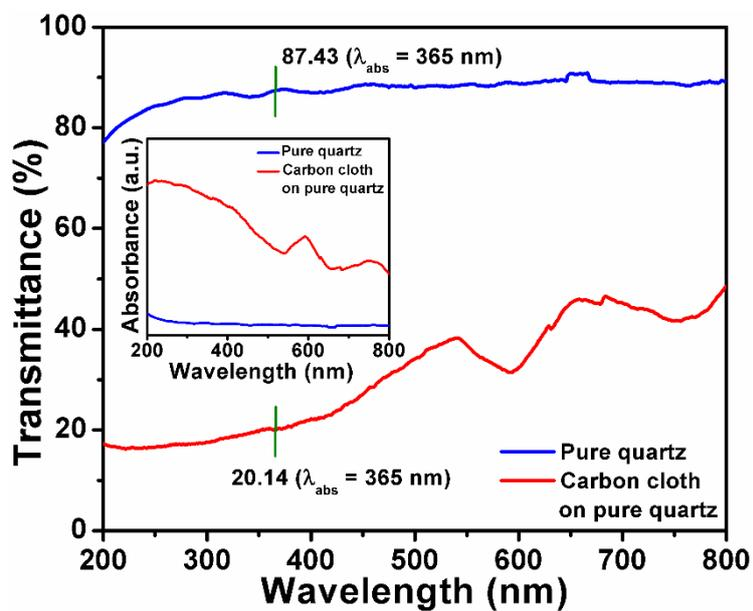
**Fig. S15.** Transmittance spectrum of carbon cloth on pure quartz. The absorbance spectrum of the corresponding transmittance is given in inset as well.
