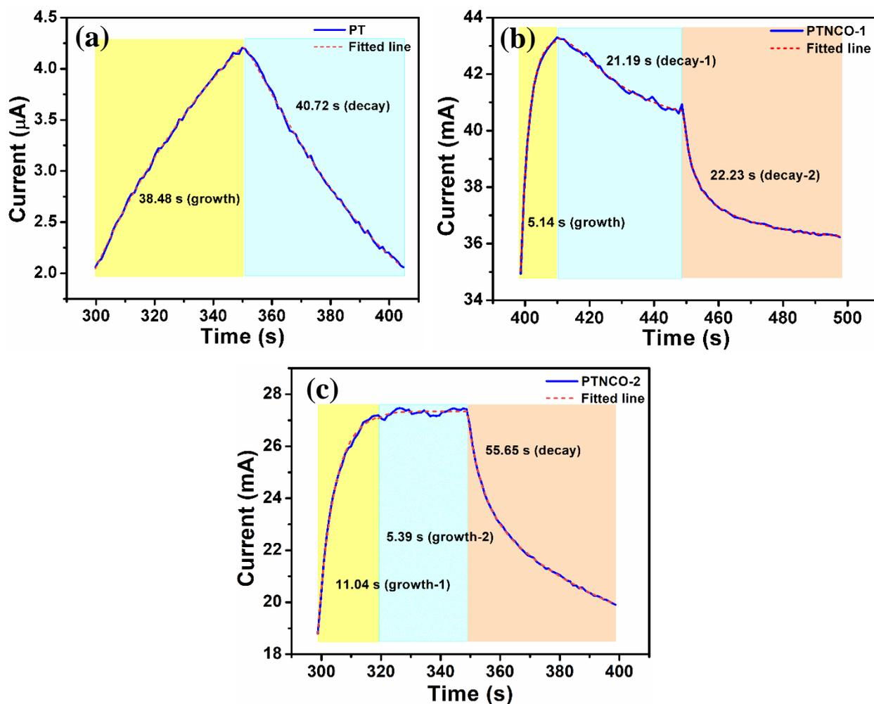
**Fig. S10.** Photo-switching curves fitted with biexponential function of equation (2) and (3) of (a) PT (b) PTNCO-1 and (c) PTNCO-2.
