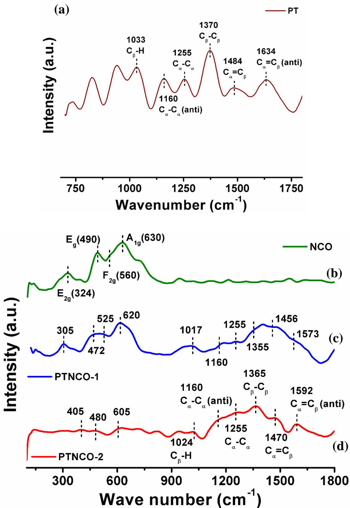
Fig. S3. RAMAN spectra of (a) NCO, (b) PT, (c) PTNCO-1 and (d) PTNCO-2.
