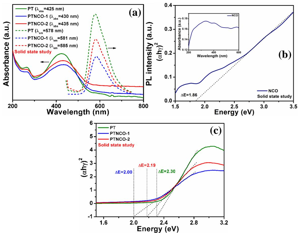
**Fig. S12.** Images of (a) UV-Vis and PL spectra of PT, PTNCO-1 and PTNCO-2, (b) Tauc plot of NCO and (c) Tauc plot of PT, PTNCO-1 and PTNCO-2 in solid state.
