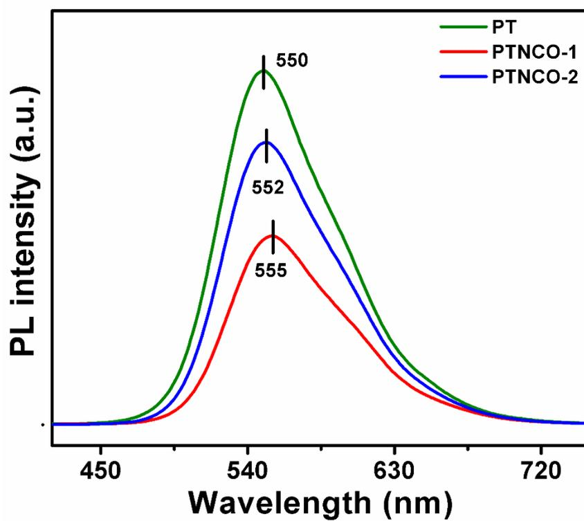
**Fig. S8.** Photo-luminescence spectrum of PT, PTNCO-1 and PTNCO-2 in THF solution.
