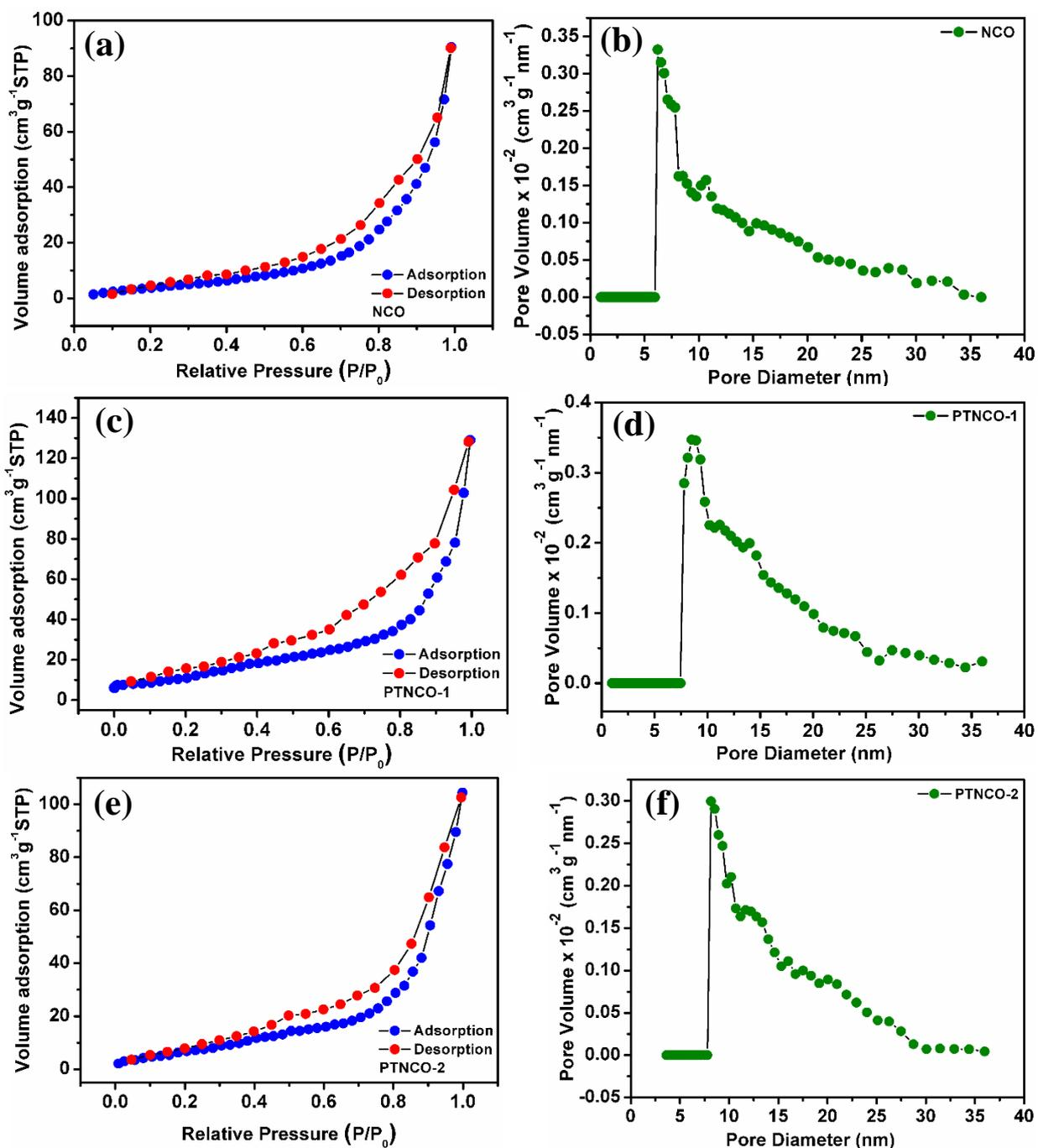
**Fig. S9.**  $N_2$  adsorption / desorption isotherms of (a) NCO, (c) PTNCO-1 and (e) PTNCO-2, pore size distribution of (b) NCO, (d) PTNCO-1 and (f) PTNCO-2 by NL-DFT method.
