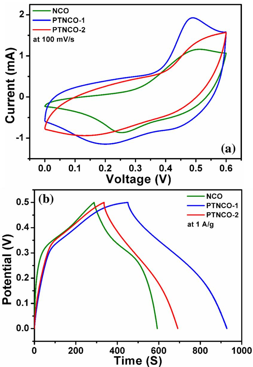
**Fig. S13.** Overlay of (a) Cyclic voltammograms of NCO, PTNCO-1 and PTNCO-2 at 100 mV/s scan rates and (b) GCD plots of NCO, PTNCO-1, and PTNCO-2 at 1 A/g current density.
