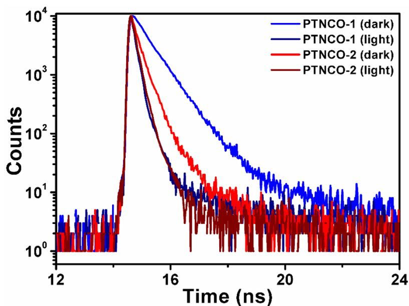
**Fig. S11.** TCSPC study of the PTNCO-1 and PTNCO-2 film before and after the irradiation of light (1 sun intensity).
