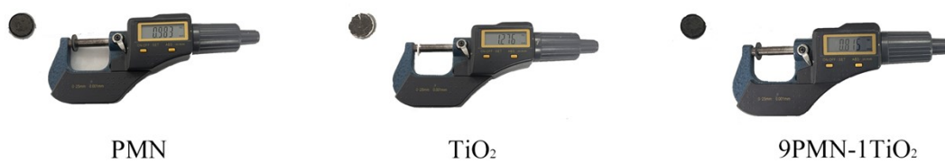
Supplementary Fig. 8 Thickness of PMN, TiO 2 and 9PMN-1TiO 2 electrolyte in DC test.
