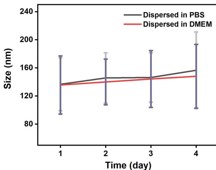
Figure S4. Changes in hydrodynamic size of  $\text{Pt/CeO}_{2-x}\text{S}_x$  suspended in PBS buffer and DMEM, respectively.
