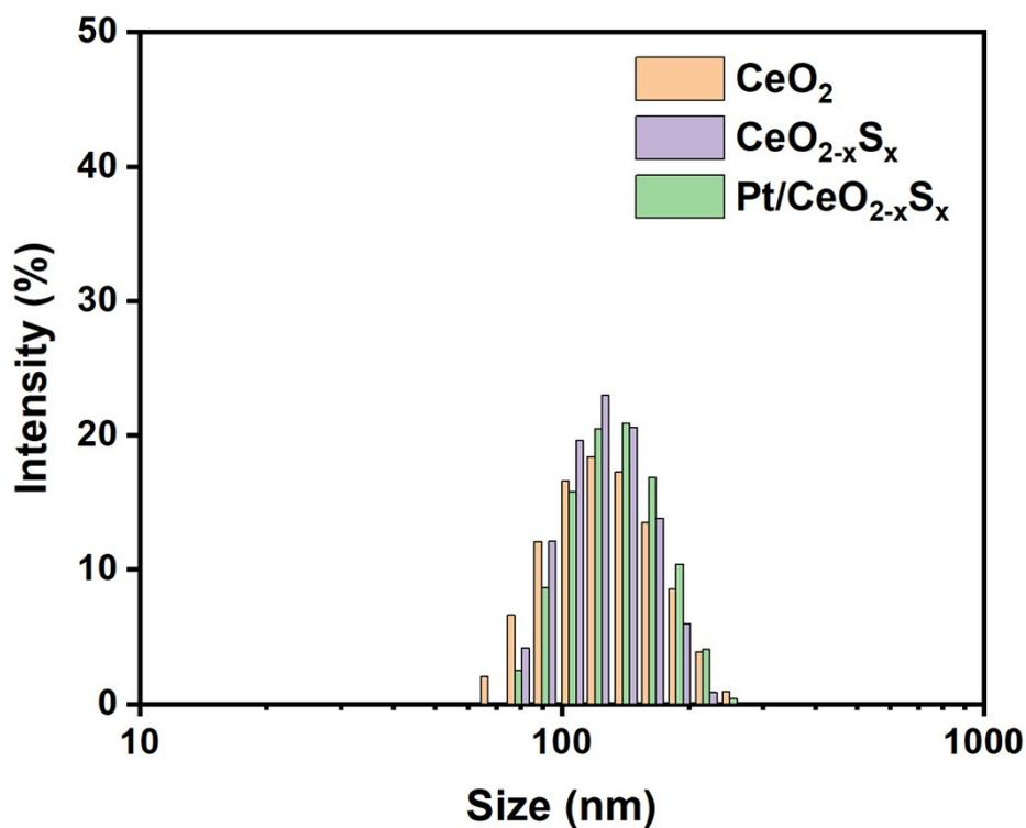
Figure S3. The size distribution of  $\text{CeO}_2$ ,  $\text{CeO}_{2-x}\text{S}_x$ , and  $\text{Pt/CeO}_{2-x}\text{S}_x$  dispersed in  $\text{H}_2\text{O}$  determined by dynamic light scattering (DLS).
