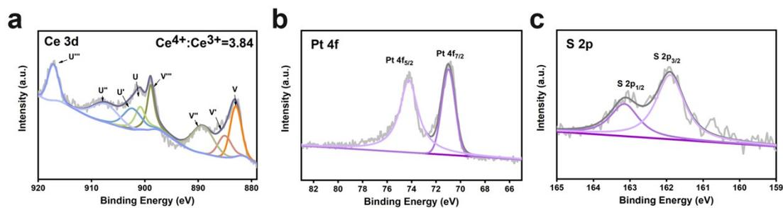
**Figure S5.** XPS spectrum of Pt/CeO<sub>2-x</sub>S<sub>x</sub>. (a) XPS spectrum of Ce 3d of Pt/CeO<sub>2-x</sub>S<sub>x</sub>. (b) XPS spectrum of Pt 4f of Pt/CeO<sub>2-x</sub>S<sub>x</sub>. (c) XPS spectrum of S 2p of Pt/CeO<sub>2-x</sub>S<sub>x</sub>.
