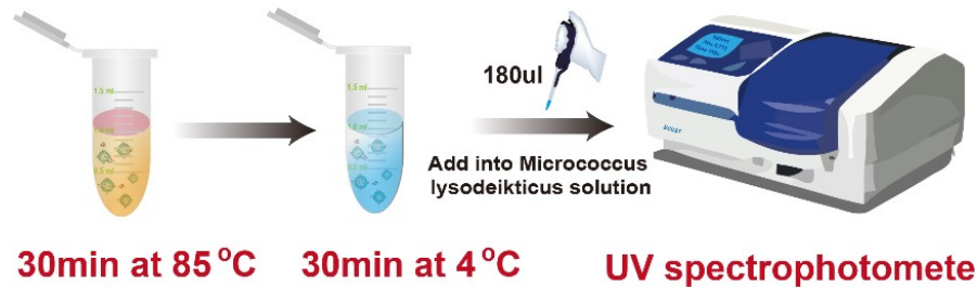
Fig. S2 Experimental diagram of relative activity measurement of heat-treated lysozyme
