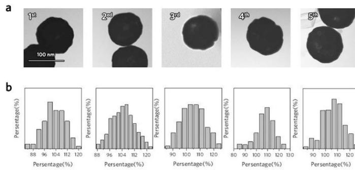
**Fig. S7** TEM images (a) and corresponding histograms (b) of AHSNs obtained after each heating and cooling cycle. The average diameters are 105.8, 104.6, 104.8, 108 and 106.2 nm, respectively.
