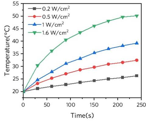
**Fig. S8** Photothermal-heating curves of AHSNs ( $10 \mu\text{g mL}^{-1}$ ) under NIR laser illumination at various laser power densities.
