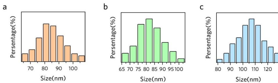
**Fig. S3** Histograms of size distribution of SNs (a), HSNs (b) and AHSNs (c), respectively.
