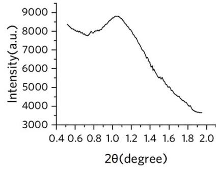
**Fig. S1 (a)** Small-angle x-ray scattering result of the obtained SNs.
