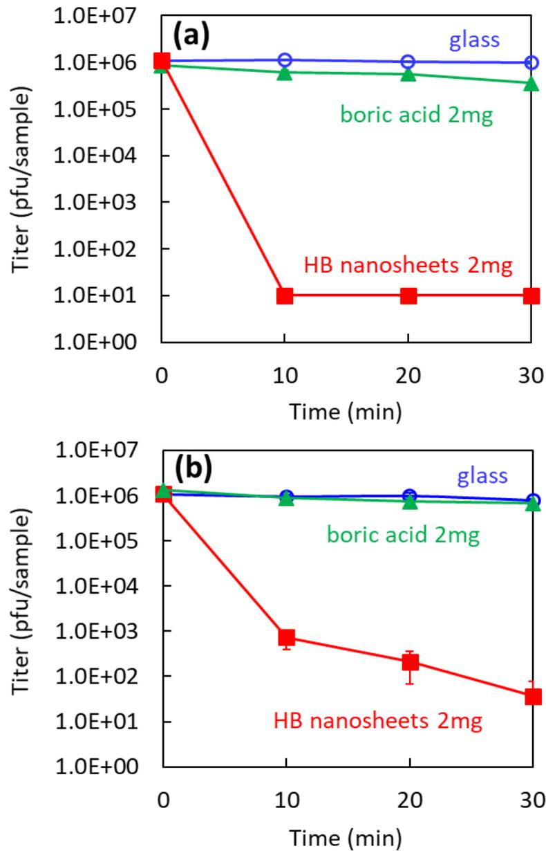
**Fig. S5.** Titer of bacteriophage  $\Phi 6$  (a) and bacteriophage  $Q\beta$  (b) as a function of exposure time to the thin film of HB nanosheets (red squares), boric acid (green triangles), a bare glass substrate (blue circles).
