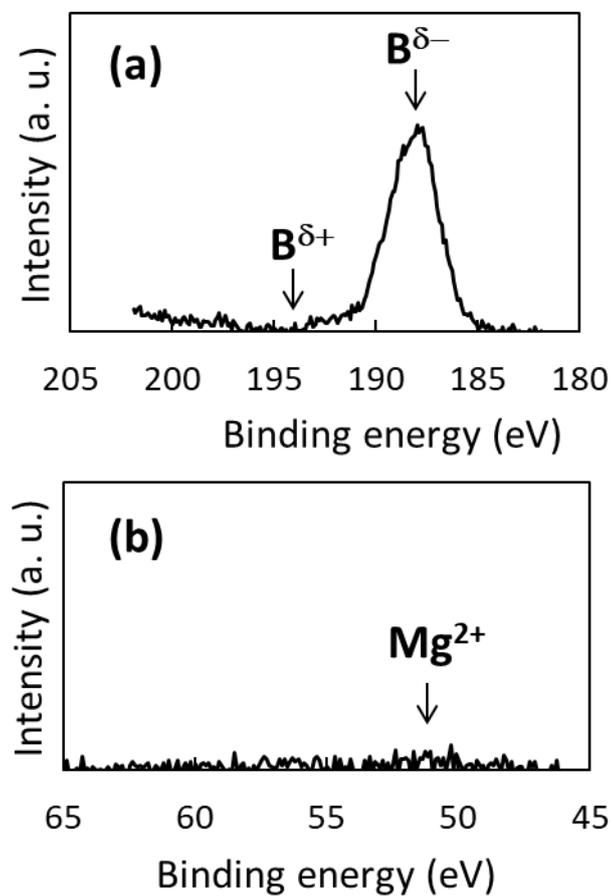
**Fig. S1.** XPS spectra of HB nanosheets for boron 1s (a) and magnesium 2p (b) orbitals.
