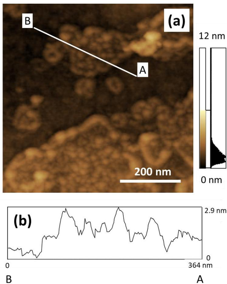
**Fig. S2.** AFM image of HB nanosheets coated on an atomically flat mica substrate (a). Panel (b) shows the height profile of the line (A-B) indicated in panel (a).
