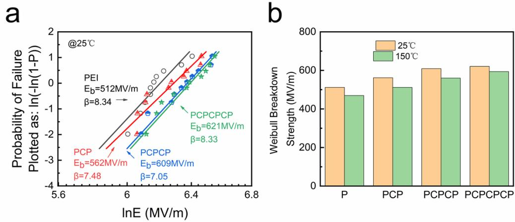
Figure S5. (a) Weibull breakdown characteristics at 25 °C. (b) Comparison of Weibull breakdown characteristics of different nanocomposites at 25 °C and 150 °C
