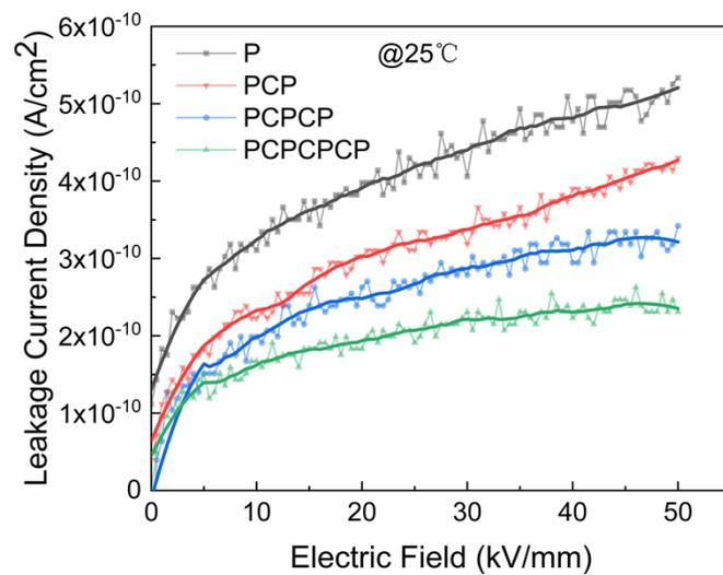
Figure S4. The leakage current for different nanocomposites at 25 °C.
