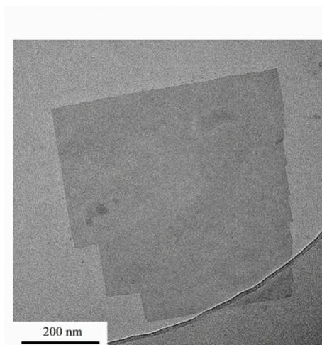
Figure S2. Transmission electron microscopy of CNO nanosheet.
