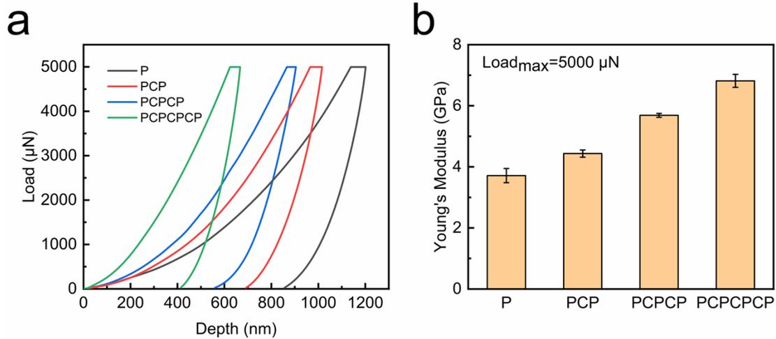
Figure S6. (a) load-displacement curves of different nanocomposite films obtained by nanoindentation.
