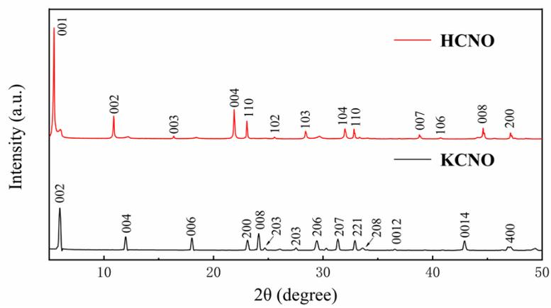
Figure S1. XRD of KCNO and HCNO Powders
