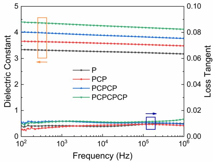
Figure S3. The dependences of dielectric constant and dielectric loss on the frequency from 100 to 1MHz at 25 °C.
