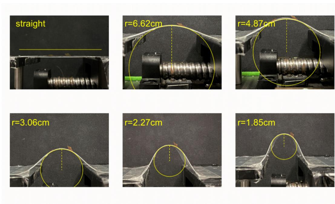
Figure S12. Actual situation of different bending degrees of nanocomposite films
