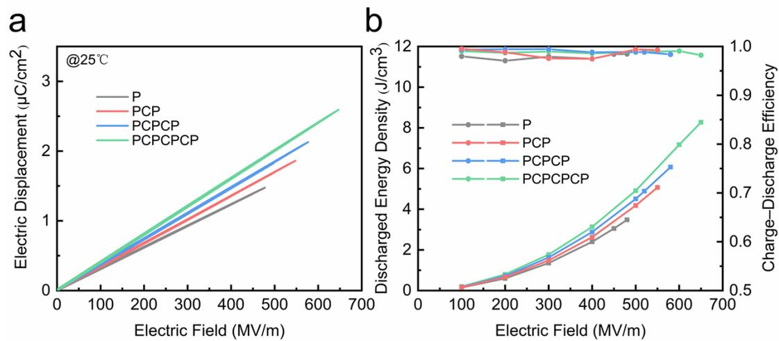
Figure S9. a) D-E loops of various nanocomposites at 25°C. b) Variation of discharged energy density and charge-discharged energy efficiency with the applied electric field for different nanocomposites at 25°C.
