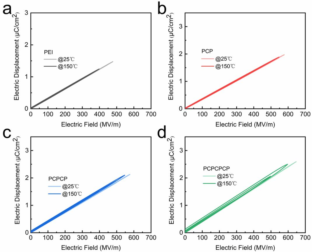
Figure S8. The comparison of D-E loops between RT and  $150^\circ\text{C}$ : (a) PEI; (b) PCP; (c) PCPCP; (d) PCPCPCP.
