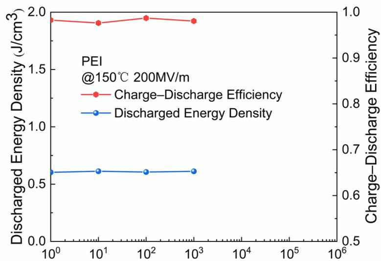
Figure S10. Discharged energy density and charge-discharged energy efficiency of PEI (at 200 MV/m) at 150 °C within 10<sup>3</sup> cycles.
