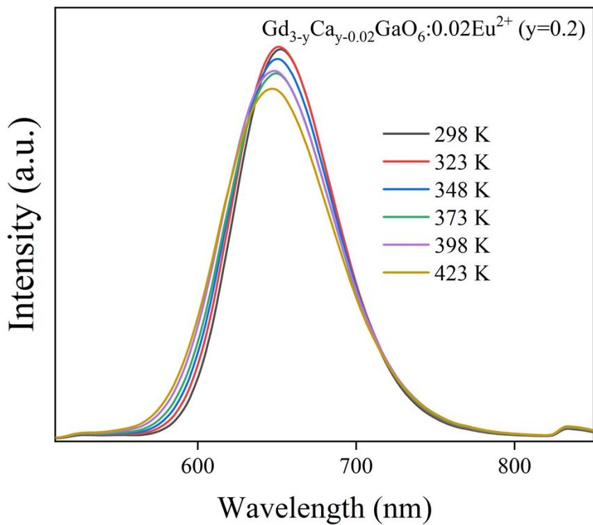
Fig. S5 Temperature-dependent PL spectra of  $\text{Gd}_{3-y}\text{Ca}_{y-0.02}\text{GaO}_6:0.02\text{Eu}^{2+}$  (y=0.2).
