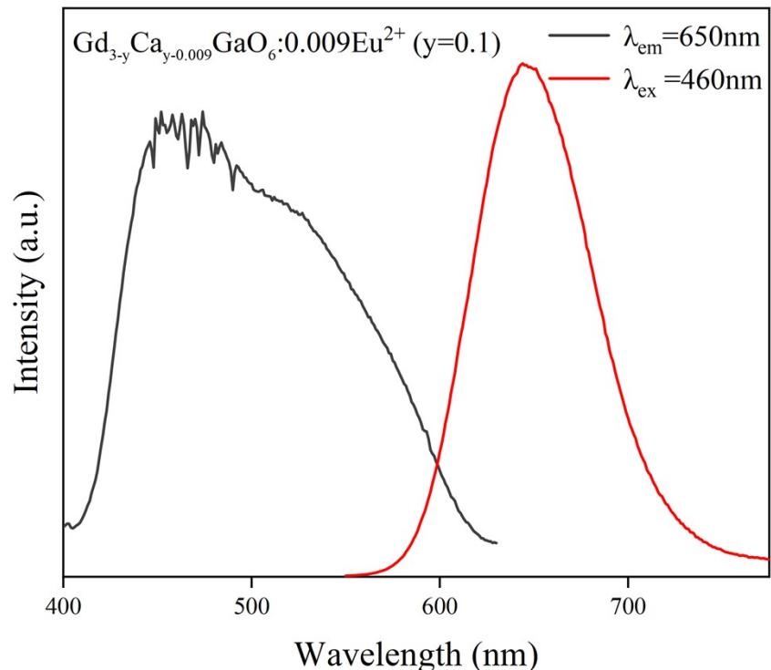
Fig. S1 PL and PLE spectra of  $\text{Gd}_{3-y}\text{Ca}_{y-0.009}\text{GaO}_6:0.009\text{Eu}^{2+}$  ( $y=0.1$ ).
