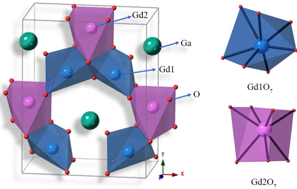
Fig. S3 Crystal structure of  $\text{Gd}_3\text{GaO}_6$ .
