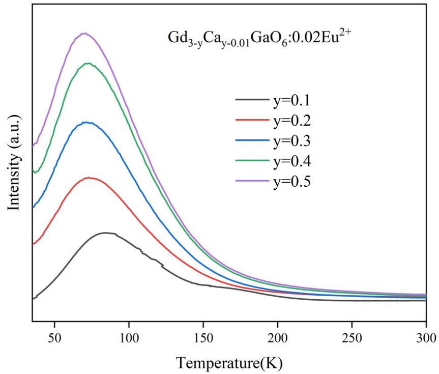
Fig. S4 TL spectra of  $\text{Gd}_{3-y}\text{Ca}_{y-0.02}\text{GaO}_6:0.02\text{Eu}^{2+}$  ( $y = 0.1-0.5$ ).
