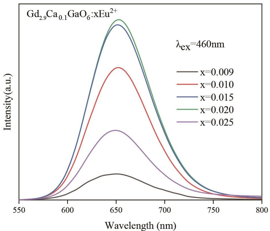
Fig. S2 PL spectra of  $\text{Gd}_{2.9}\text{Ca}_{0.1}\text{GaO}_6:x\text{Eu}^{2+}$  ( $x = 0.009-0.025$ ).
