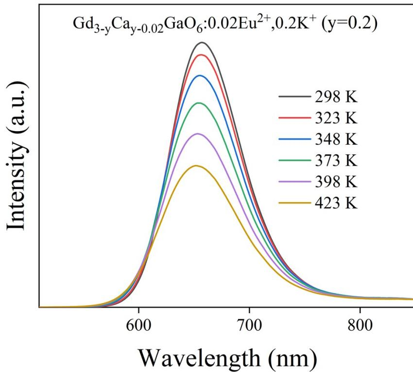
Fig. S6 Temperature-dependent PL spectra of  $\text{Gd}_{3-y}\text{Ca}_{y-0.02}\text{GaO}_6:0.02\text{Eu}^{2+}, 0.2\text{K}^+$
