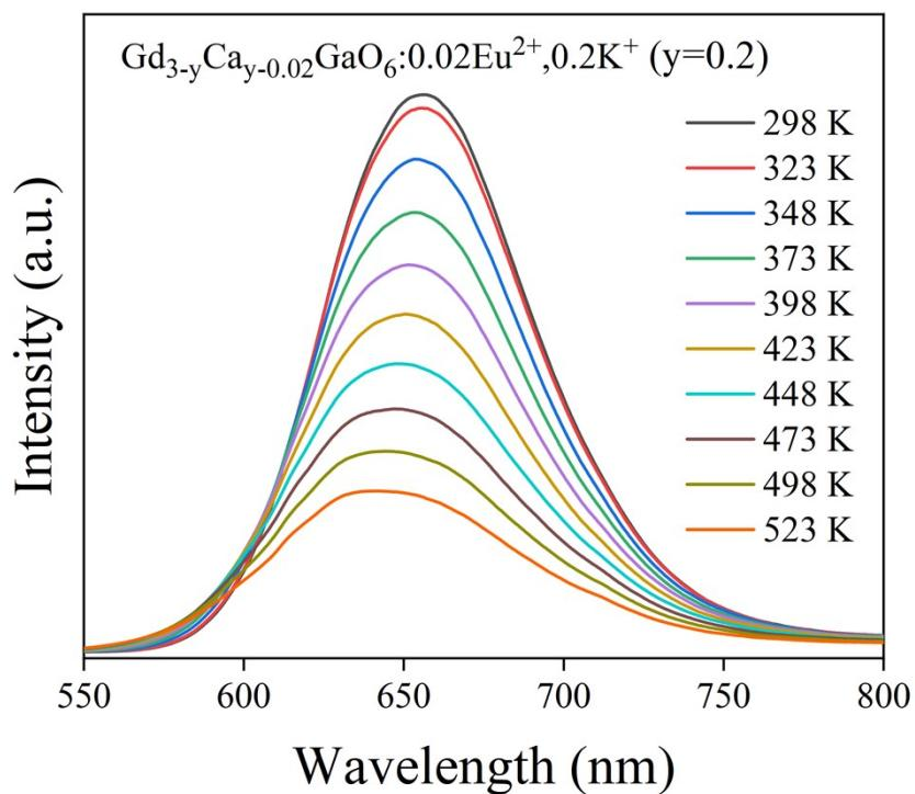
Fig. S8 Temperature-dependent PL spectra of  $\text{Gd}_{3-y}\text{Ca}_{y-0.02}\text{GaO}_6:0.02\text{Eu}^{2+}, 0.2\text{K}^+$
