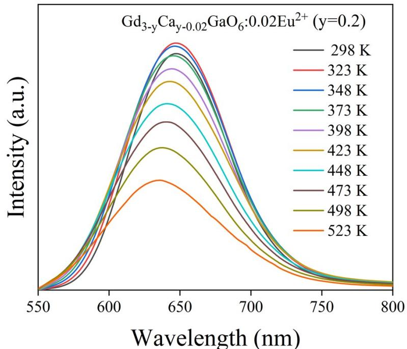
Fig. S7 Temperature-dependent PL spectra of  $\text{Gd}_{3-y}\text{Ca}_{y-0.02}\text{GaO}_6:0.02\text{Eu}^{2+}$  (y=0.2).
