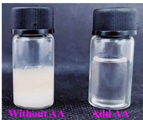
Figure S3. The photos of the CPU-5 without and with the addition of AA.
