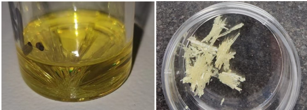
Figure S3. \text{FA}_3\text{BiBr}_6 crystals growth at 75\text{ }^\circ\text{C} and crystals after vacuum drying.
