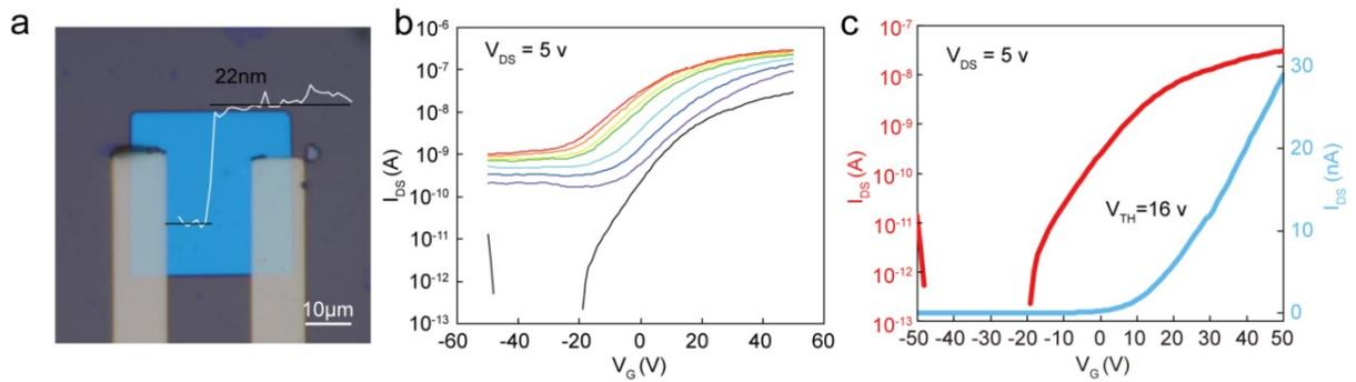
**Figure S8.** (a) Optical image of BiOI-based photodetectors. (b) The  $I_D$ - $V_G$  curve of photocurrent controlled by  $\text{SiO}_2$  as backgate. (c) Transfer curve of the BiOI FET,  $V_D = 5$  V.
