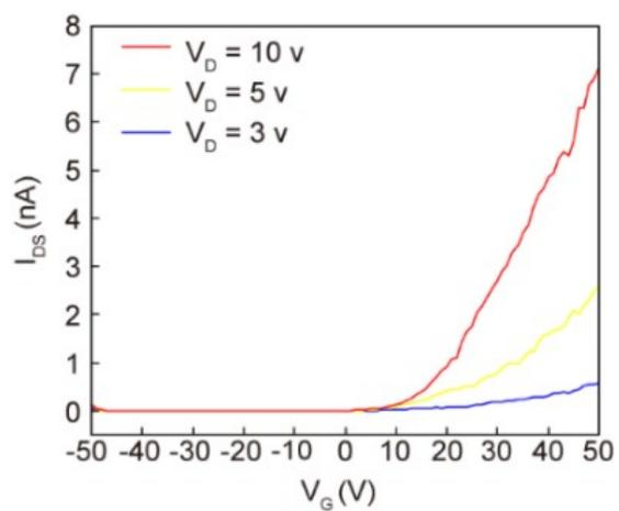
**Figure S4.**  $I_D$ - $V_G$  curves of BiOI/SiO<sub>2</sub> transistors at different source-drain voltages, the n-type characteristics of BiOI were demonstrated.
