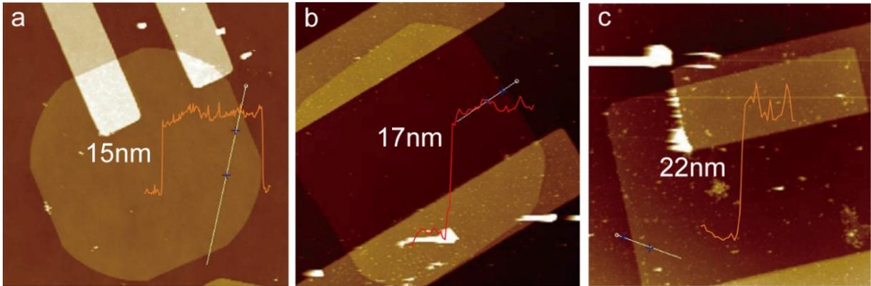
**Figure S5.** AFM images of BiOI devices of different thicknesses.
