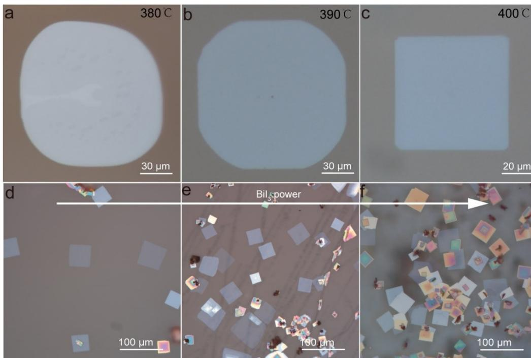
**Figure S1.** Growth regulation of BiOI nanosheets on mica. (a, b, c) BiOI nanosheets with different morphologies were grown at 380 °C, 390 °C and 400 °C. (d, e, f) Different morphologies of BiOI nanosheets grown from low to high BiI<sub>3</sub> concentrations.
