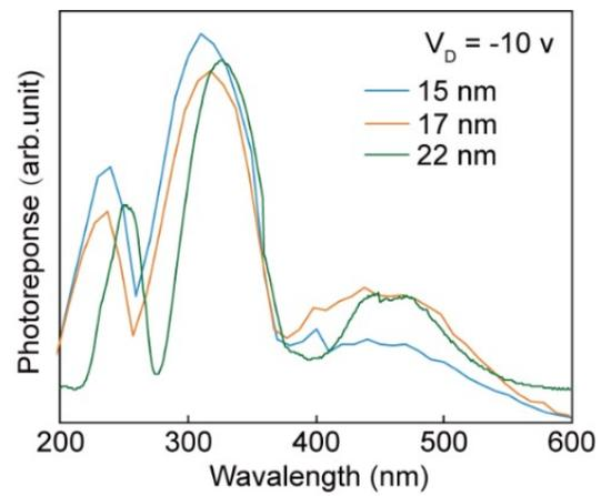
**Figure S6.** Optical response spectra of BiOI nanosheets with different thicknesses at 400  $\mu\text{W cm}^{-2}$  power density under irradiation at different wavelengths.
