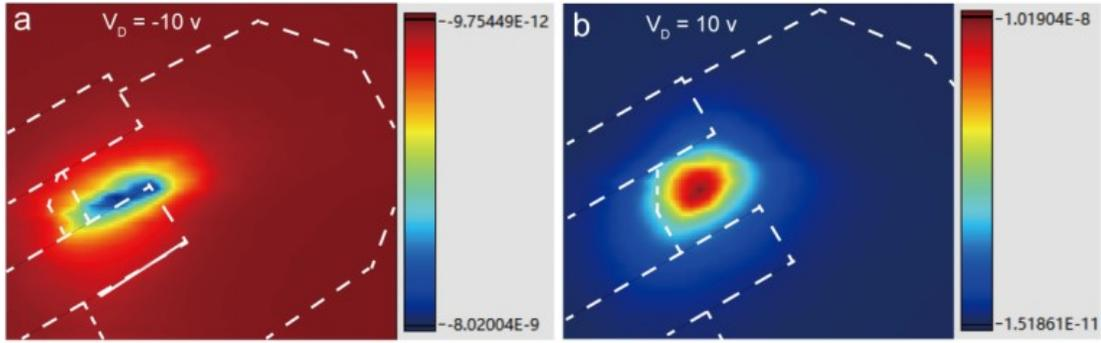
**Figure S7.** Scanning photocurrent mapping of the BiOI device under 405 nm laser illumination: (a)  $V_D = -10$  V and (b)  $V_D = 10$  V. The white dashed lines correspond to the outlines of BiOI and the electrodes.
