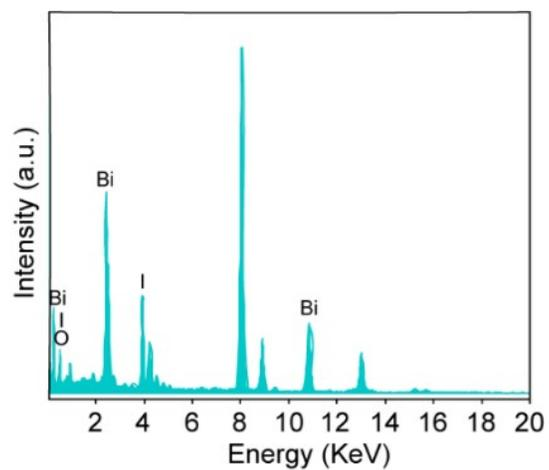
**Figure S3.** The energy-dispersive X-ray spectroscopy (EDS) of BiOI nanosheet.
