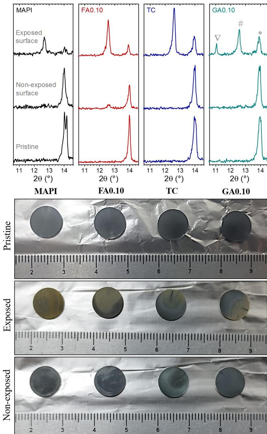
Figure S3 - Results of XRD (top) and visual aspect of samples (down) in pristine and after thermal treatment at 200 °C for 4 h conditions in the exposed and non-exposed surfaces. Peak assignments are  $\nabla$ : GAPbI<sub>3</sub>, #: PbI<sub>2</sub>, and \*: perovskite. Yellowing of the exposed surfaces are due to formation of PbI<sub>2</sub>, which was barely formed at the non-exposed surfaces of the same samples.
