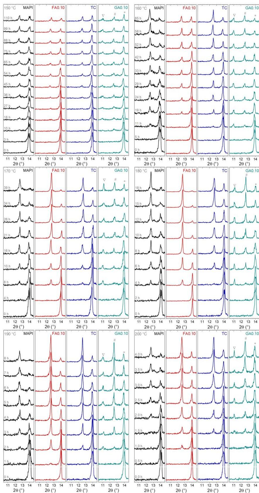
Figure S1 - X-ray diffraction of the first set of studied compositions at different times and temperatures of thermal treatment. Peak assignments are ▽: GAPbI<sub>3</sub>, #: PbI<sub>2</sub>, and \*: perovskite.
