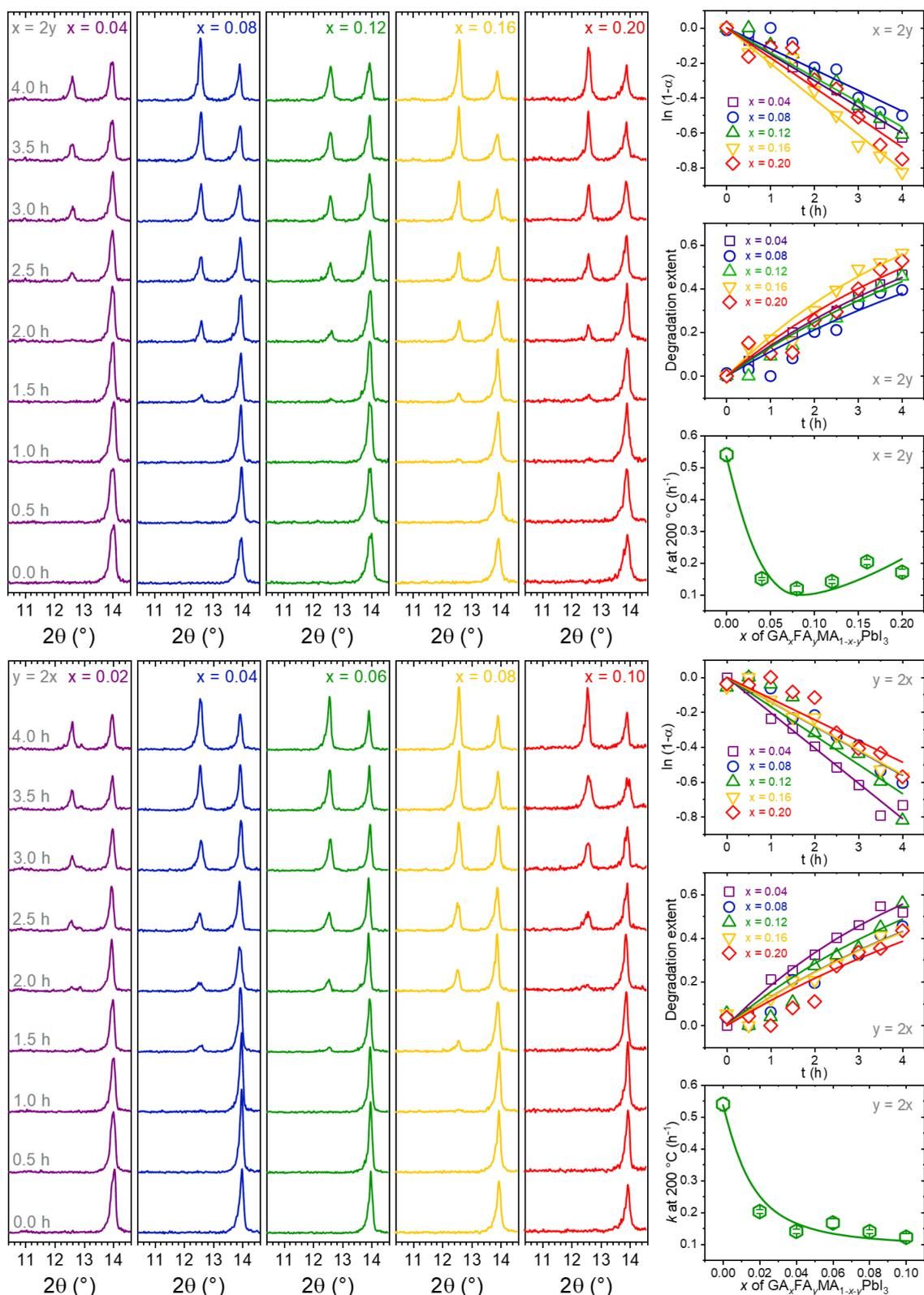
Figure S5 - Thermal degradation data and results of  $\text{GA}_x\text{FA}_y\text{MA}_{1-x-y}\text{PbI}_3$  perovskites for the set of compositions  $x = 2y$  (top) and  $y = 2x$  (bottom).
