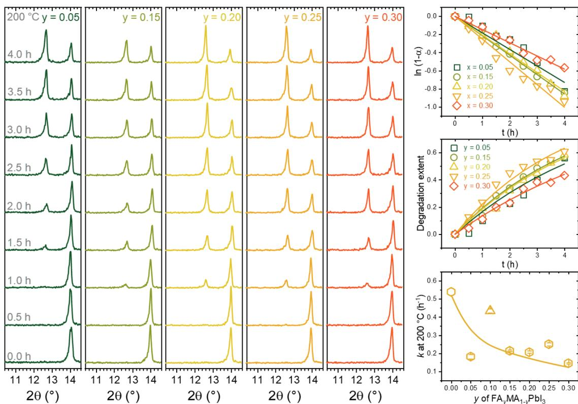
Figure S6 - Thermal degradation data and results of  $\text{FA}_y\text{MA}_{1-y}\text{PbI}_3$  perovskites.
