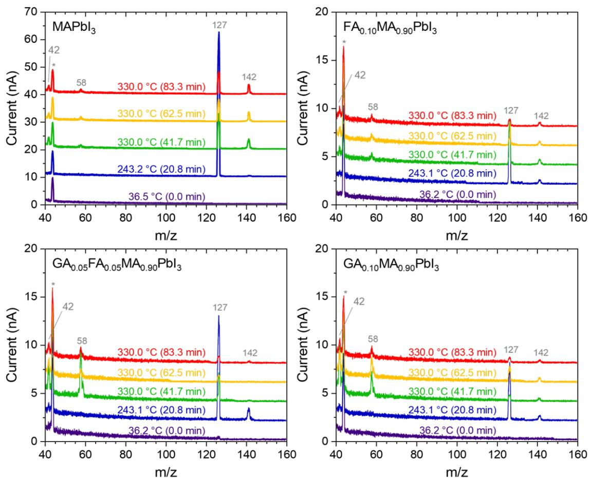
Figure S4 - Instant mass spectra in the  $m/z$  range from 40 to 160 collected at different times. The peak at  $m/z = 44$  (\*) is due to the pulsed  $\text{CO}_2$  injections used for calibration. Vertical shifts between spectra were made intentionally for better visualization of results.
