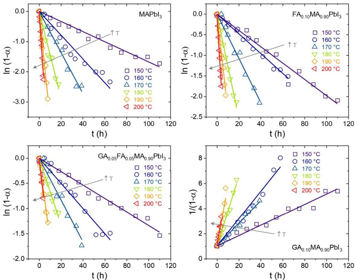
Figure S2 - Experimental data and linear fits at different temperatures for MAPI, FA0.10, TC, and GA0.10.
