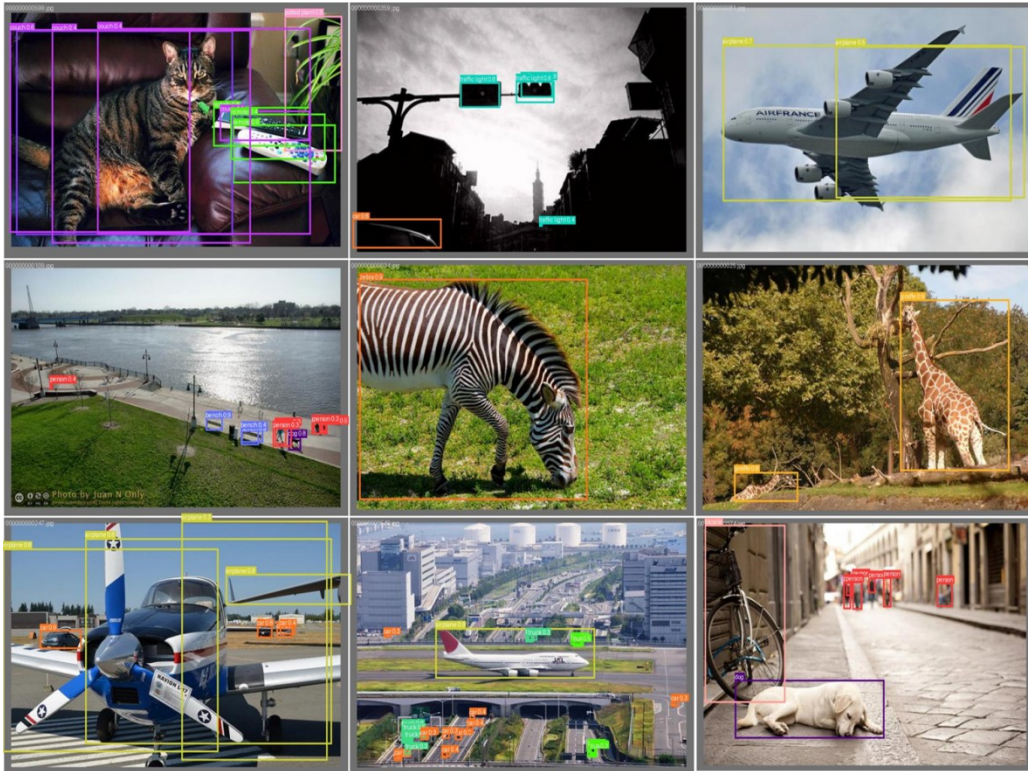
Fig.S11. Recognition effect diagram of YOLO network. The prediction box is the object we tracked. The prediction box shows the type of object identified and the probability of accurate recognition.
