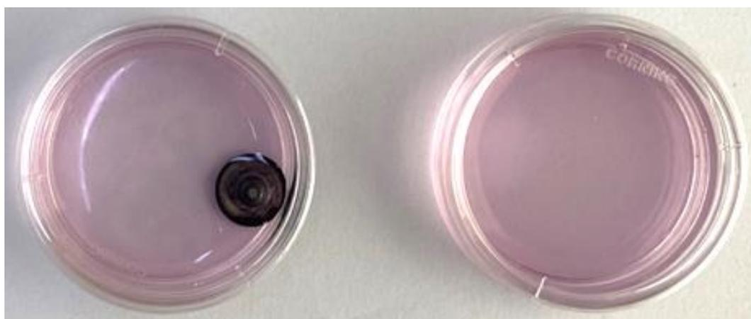
**Fig. S35.** Photograph of L929 cells cultured in environments with and without Au-FLG electrode.
