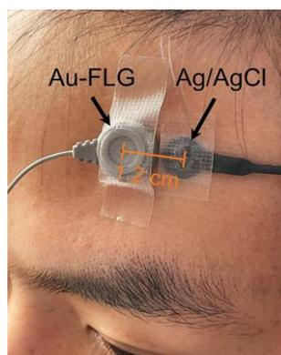
**Fig. S17.** Position of Au-FLG and Ag/AgCl electrodes on the scalp (Fp1).
