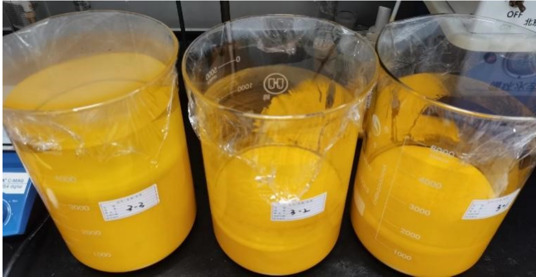
Fig. S1. The photograph of PbI 2 production at kilogram class.
