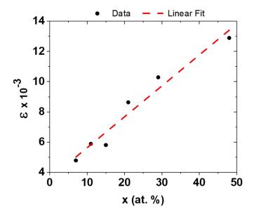
**Supplementary Figure 1.** Microstrain as a function of the Fe at. %. Experimental data in black circles and linear fit in dashed red line.
