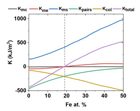
**Supplementary Figure 2.** Dependency of the different magnetic anisotropies with respect to Fe content (at.%). In this figure, columnar growth is considered as a source of OOP anisotropy. The dashed line at Fe 19 at.% indicates the change of sign in  $K_{tot}$ .
