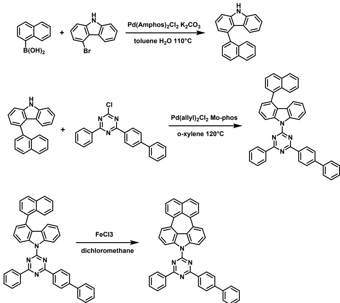
Fig. S1 The synthesis route and method for Hept-TRZ
