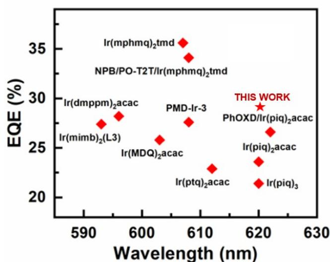
Fig. S7 Summary of existing phosphorescent OLED technologies
