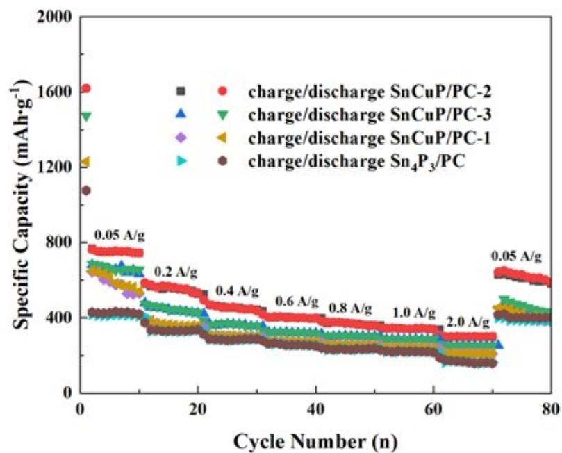
Fig. S6 Rate performance of SIBs with  $\text{SnCuP}/\text{PC-X}$ ;
