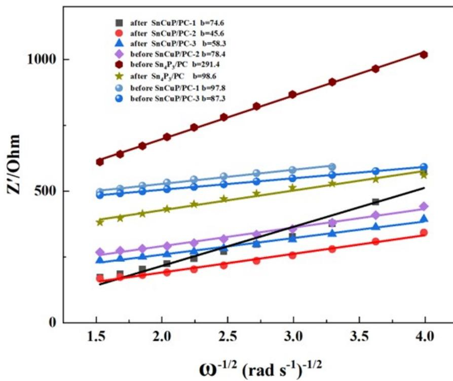
Fig. S11 The relationship between  $Z'$  and  $\omega^{-1/2}$  of the SIB with SnCuP/PC-X in low frequency region.
