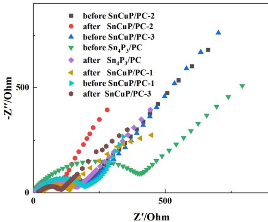
Fig. S10 Nyquist plots of the SIB with SnCuP/PC-X before and after 300 cycles.
