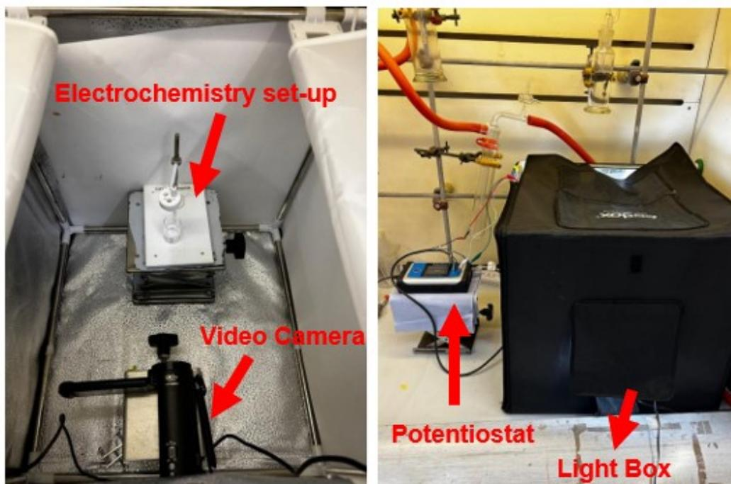
**Figure S9:** Annotated camera set-up within lightbox (left) and full experimental set-up (right) as it appeared during experiments.
