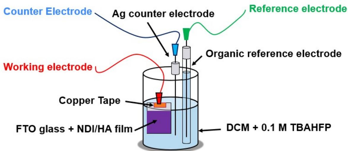
*Figure S8: Schematic of electrochemistry set-up.*
