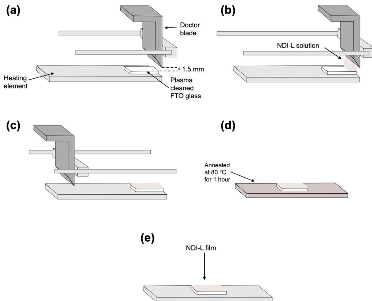
**Figure S7:** Overview of thin film casting on FTO glass using doctor blade, showing (a) calibration and set-up of the doctor blade, (b) addition of NDI solution, (c) casting of solution across glass surface, (d) thermal annealing of solution to glass, and (e) the completed NDI film.
