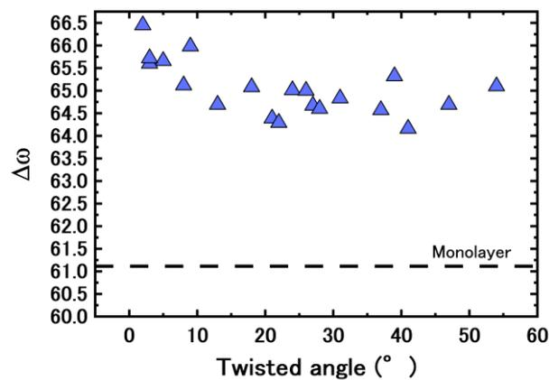
**Figure S11.** Distance in between ( $\Delta\omega$ ) A1g and E2g modes in monolayer and bilayer WS<sub>2</sub> with different twist angles.
