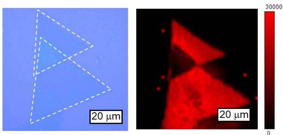
**Fig. S6.** PL intensity mapping of bilayer WS<sub>2</sub> with a twist angle of 57 degrees.
