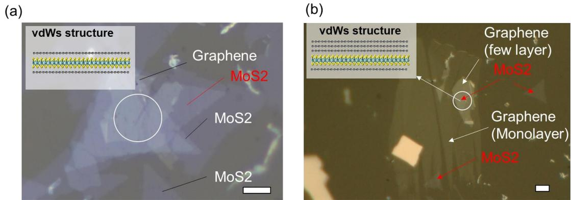
**Fig. S3.** assembly of vdWs using CVD synthesized MoS2 and mechanically exfoliated graphene. The structure of the vdWs stacking is shown in the inset. Scale bar is 30 μm.
