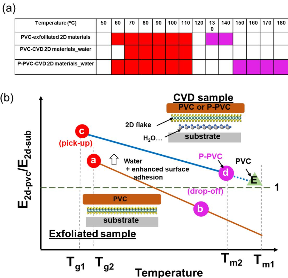
**Fig. S8.** (a) Temperature parameters of the transfer, including pick-up (red region) and drop-off (purple region), and the (b) corresponding expected adhesion variation between 2D materials /PVC stamp ( $E_{2d-PVC}$ ), and between 2D materials/substrate ( $E_{2d-sub}$ ) under various temperatures with two different experimental setups.
