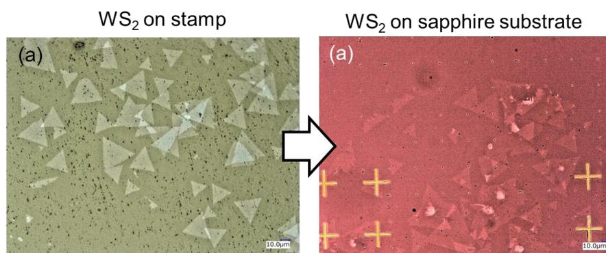
**Fig. S2.** (a) Pick up WS<sub>2</sub> in sequence and assemble the twist bilayer structure on the P-PVC stamp. (b) drop off the twist bilayer WS<sub>2</sub> on a sapphire substrate.
