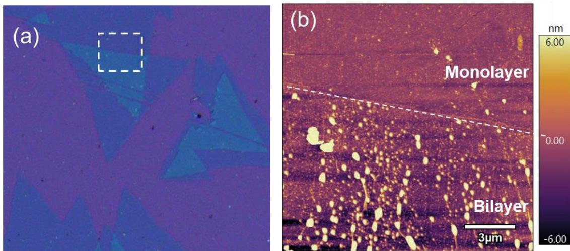
**Fig. S4.**(a) Optical and (b) AFM image of twisit bilayer WS<sub>2</sub> sample transferred on SiO<sub>2</sub> substrate. The dashed square in (a)(c) indicate the location of the AFM measurement. The monolayer region is clean, indicates little residual of PVC after transfer and cleaning, while some bubbles and wrinkles appear at the bilayer region, which is strongly influenced by the the transferring circumstance and quality of 2D material.
