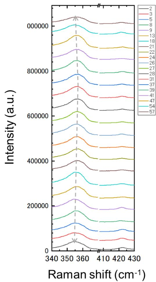
**Fig. S7.** Raman spectrum of bilayer WS<sub>2</sub> with twist angle from 2 to 57 degrees.
