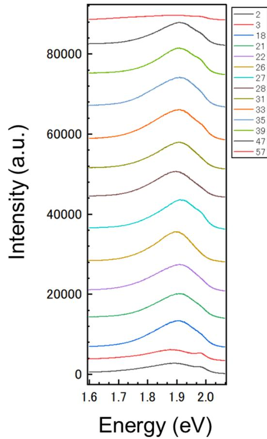
**Fig. S5.** PL spectrum of bilayer WS<sub>2</sub> with twist angle from 2 to 57 degrees.
