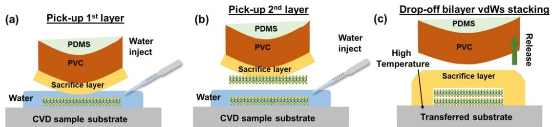
**Figure S10.** Schematic of the assembly of multi-layer vdW stacking using P-PVC.
