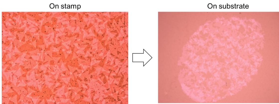
**Figure S12.** The pick-up of WS2 and that dropped off on to substrate.
