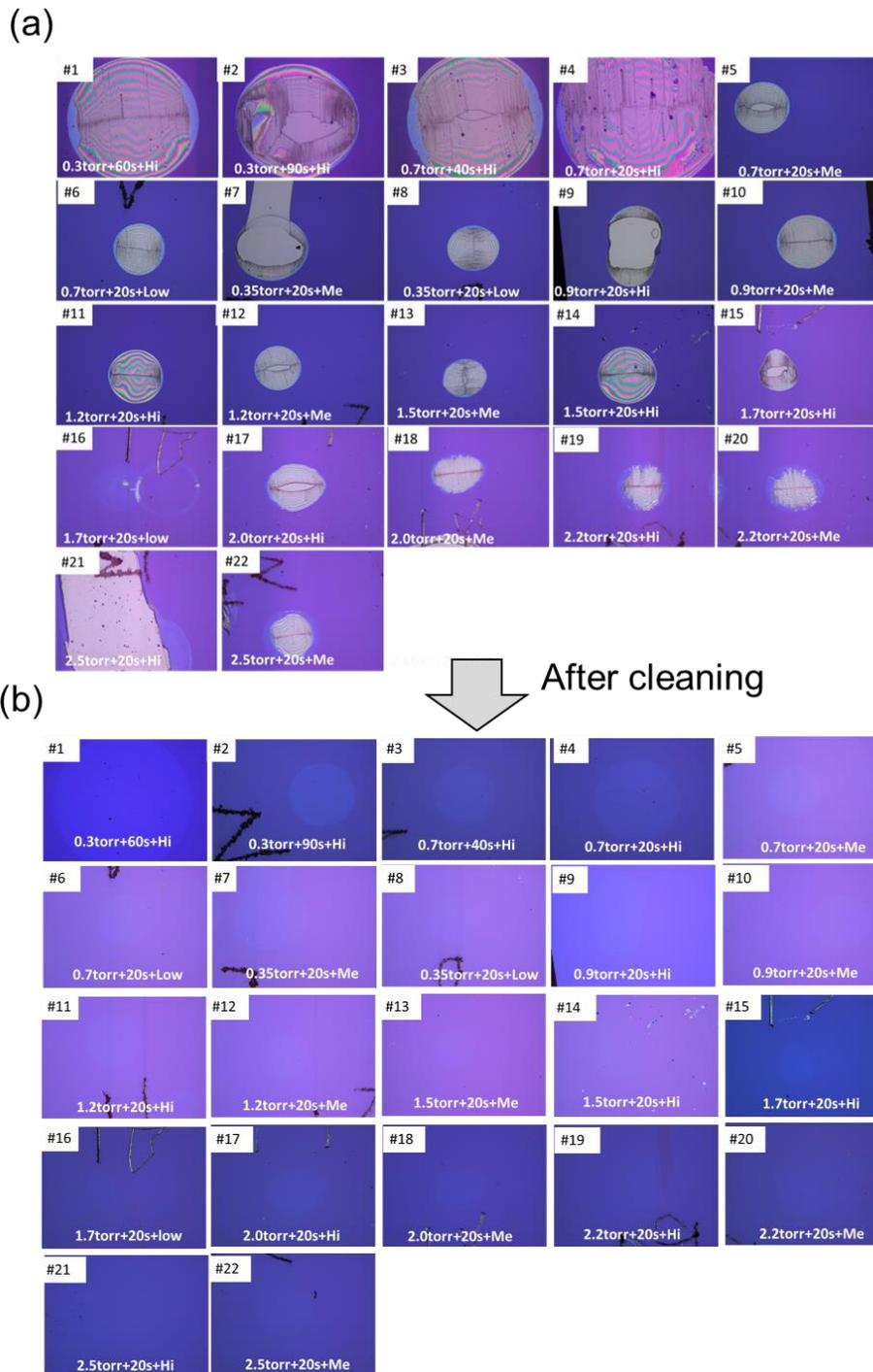
**Fig. S9.** the optical image of PVC residual (a) before and (b) after the cleaning with P-PVC treated under different plasma condition. (Low, Me, and Hi represent the plasma power, which is 6.8 W, 10.5 W, and 18 W, respectively)
