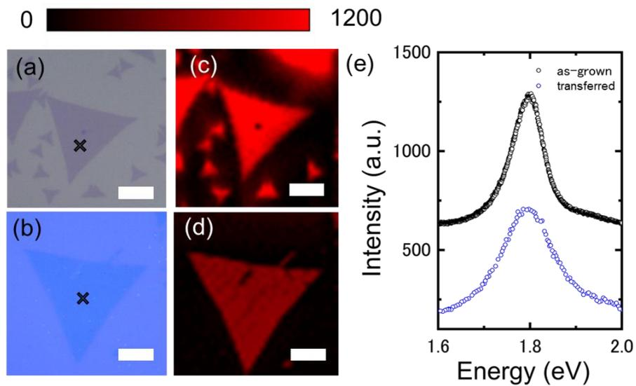
**Fig. S1.** The (a)(b)optical image, the (c)(d) PL intensity mapping and the (e) corresponding PL spectrum at the marked location of monolayer MoS<sub>2</sub> before (on SiO<sub>2</sub>) and after transfer by P-PVC (on SiO<sub>2</sub>), respectively. Scale bar is 20 μm.
