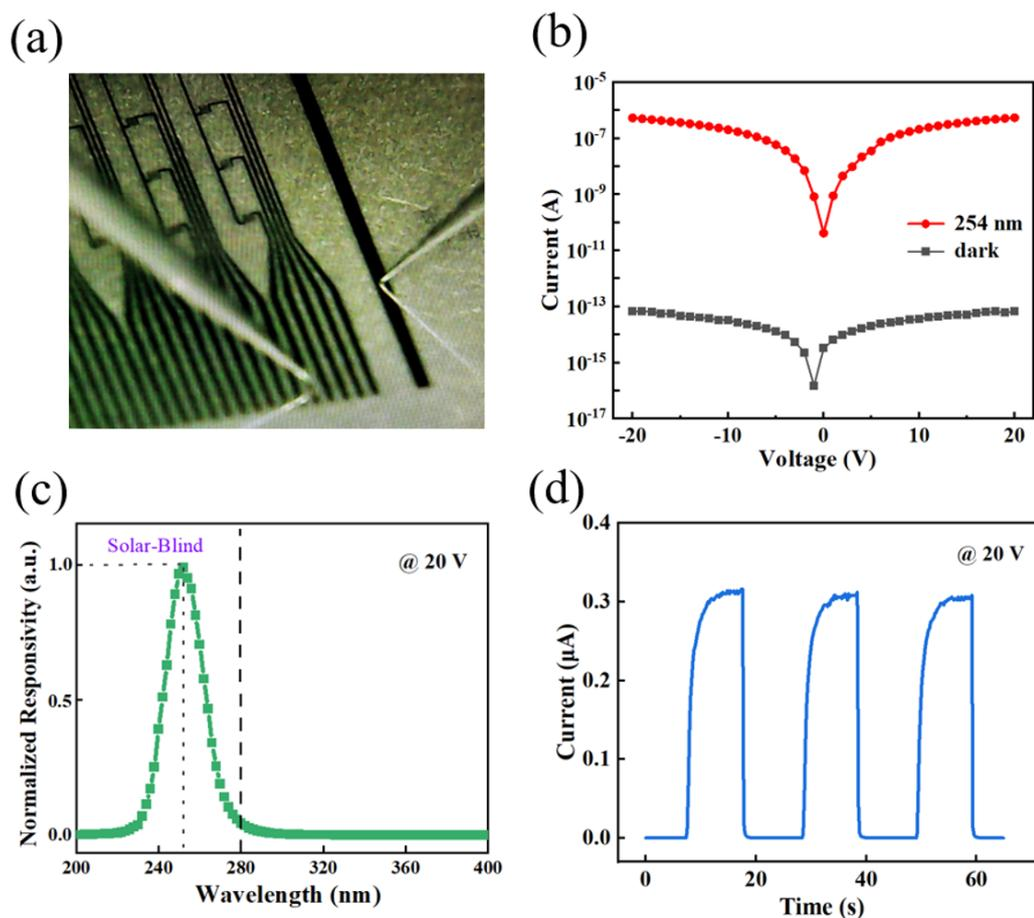
**Figure S5.** (a) Performance testing image of a single device in the photodetector array; (b) I-V characteristic curves of a single device in the photodetector array in the dark and under 254 nm UV illumination; (c) Normalized spectral response curve of a single device in the photodetector array at a bias voltage of 20 V; and (d) Multi-cycle I-T characteristic curves of a single device in the photodetector array at a bias voltage of 20 V.
