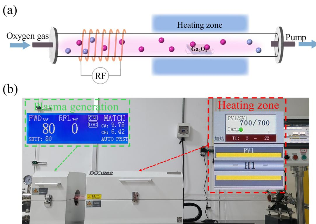
**Figure S1.** (a) Schematic diagram and (b) photograph of the remote plasma enhanced chemical vapor deposition system.
