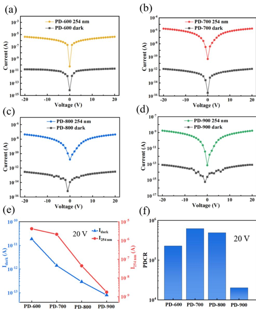
**Figure S2.** I-V characteristic curves of (a) PD-600, (b) PD-700, (c) PD-800, and (d) PD-900 in the dark and under 254 nm UV illumination; (e) Summary chart of the photocurrent and dark current at a bias of 20 V; and (f) Summary chart of the photo-to-dark current ratio (*PDCR*) at a bias of 20 V.
