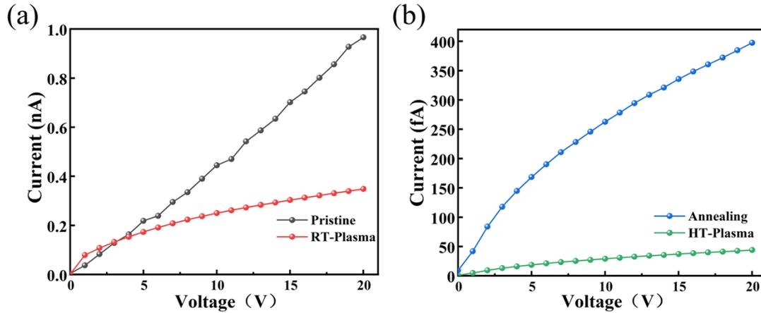
**Figure S4.** I-V curves of the MSM structured photodetectors based on (a) Pristine and RT-Plasma samples, (b) Annealing and HT-Plasma samples.
