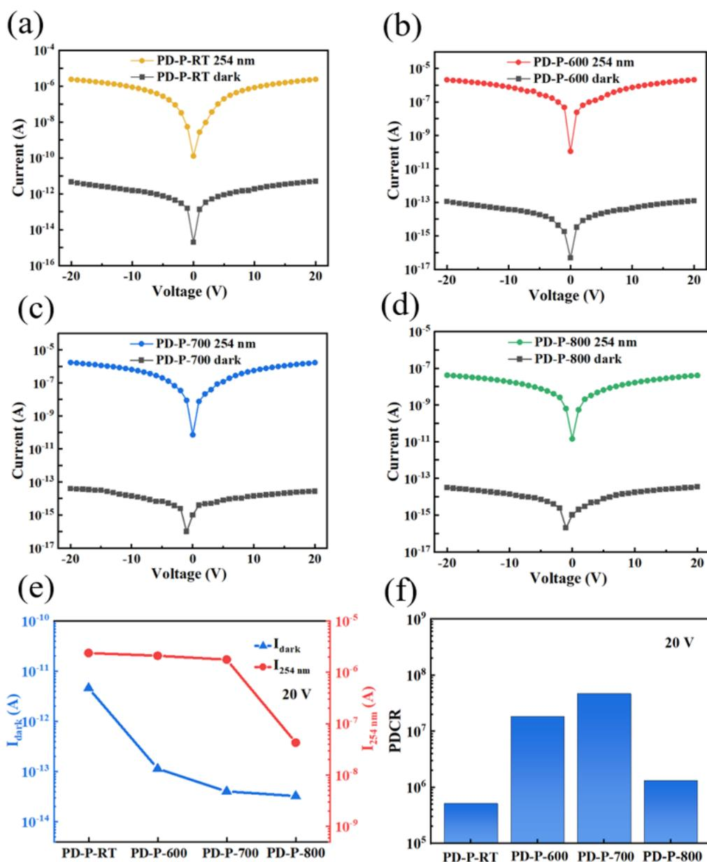
**Figure S3.** I-V characteristic curves of (a) PD-P-RT, (b) PD-P-600, (c) PD-P-700, and (d) PD-P-800 in the dark and under 254 nm UV illumination; (e) Summary chart of the photocurrent and dark current at a bias of 20 V; and (f) Summary chart of the photo-to-dark current ratio (*PDCR*) at a bias of 20 V.
