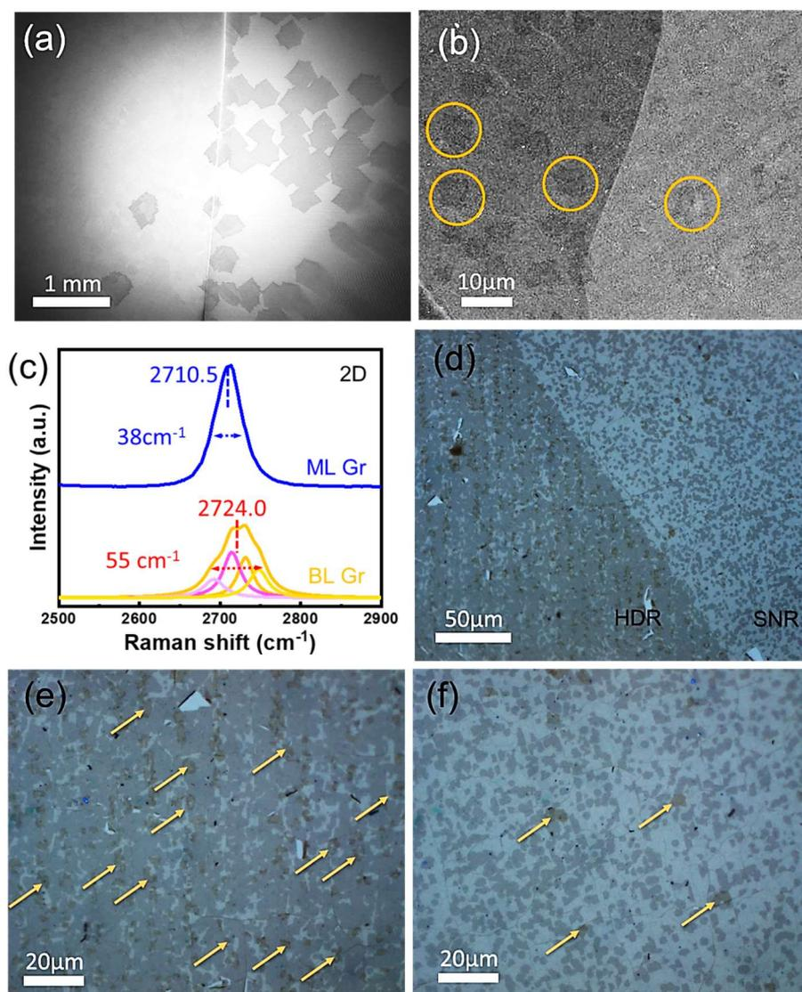
**Figure S1.** (a) SEM image of single crystal graphene synthesized on different Cu grains. (b) The distribution of adlayer graphene, highlighted by orange circles, on different Cu grains. (c) Comparison of Raman 2D band in monolayer and adlayer graphene. (d-f) Optical images of SnS<sub>2</sub> grown in HDR and SNR. The distribution of adlayer graphene, marked with yellow arrows, in (e) HDR and (f) SNR regions, respectively.
