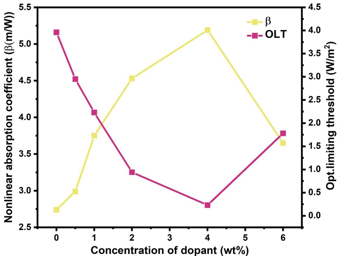
**Figure S 7:** Correlation graph of nonlinear absorption coefficient and optical limiting threshold value with concentration of boron doping
