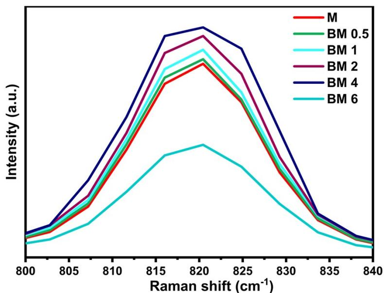
**Figure S 3:** Raman spectra peak corresponding to vibrational mode at  $818\text{cm}^{-1}$  of pristine and doped  $\text{MoO}_3$  (for finding the phonon profile)
