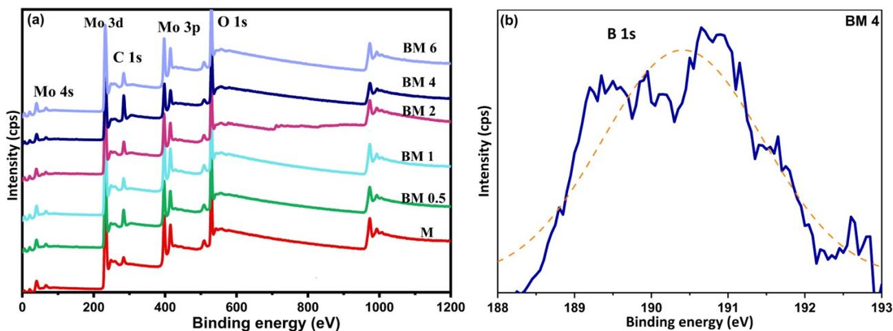
**Figure S 2:** (a) Full range XPS survey of  $\text{MoO}_3$  and B- $\text{MoO}_3$  samples (b) B 1s spectra of BM 4 sample
