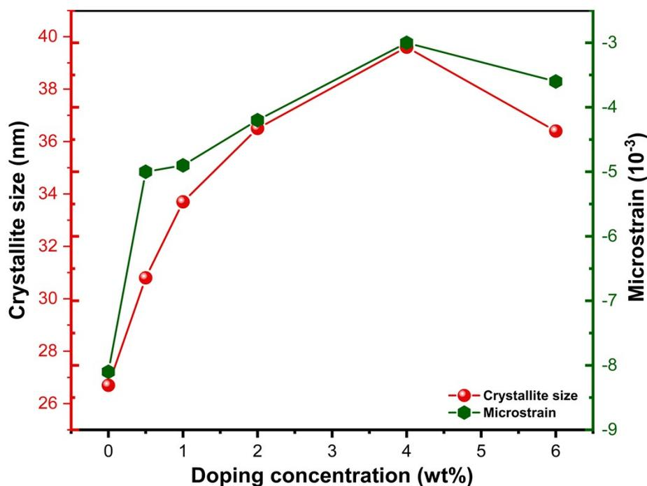
**Figure S 1:** Correlation graph of crystallite size and microstrain with doping concentration of boron
