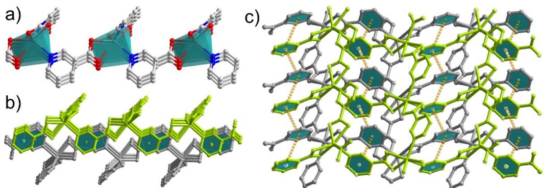
**Figure S8.** a) 2D framework structure of SUST-P3. b, c) Intermolecular  $\pi$ - $\pi$  interactions in SUST-P3.
