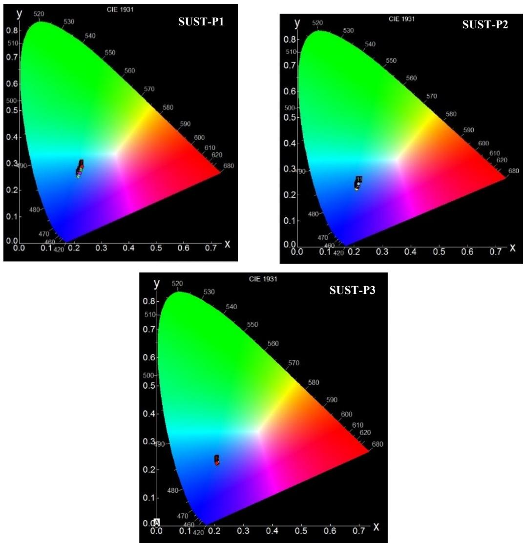
**Figure S16.** CIE coordinates corresponded to temperature-dependent prompt emissions of SUST-P1, SUST-P2 and SUST-P3 from 77 to 300 K in solid state.
