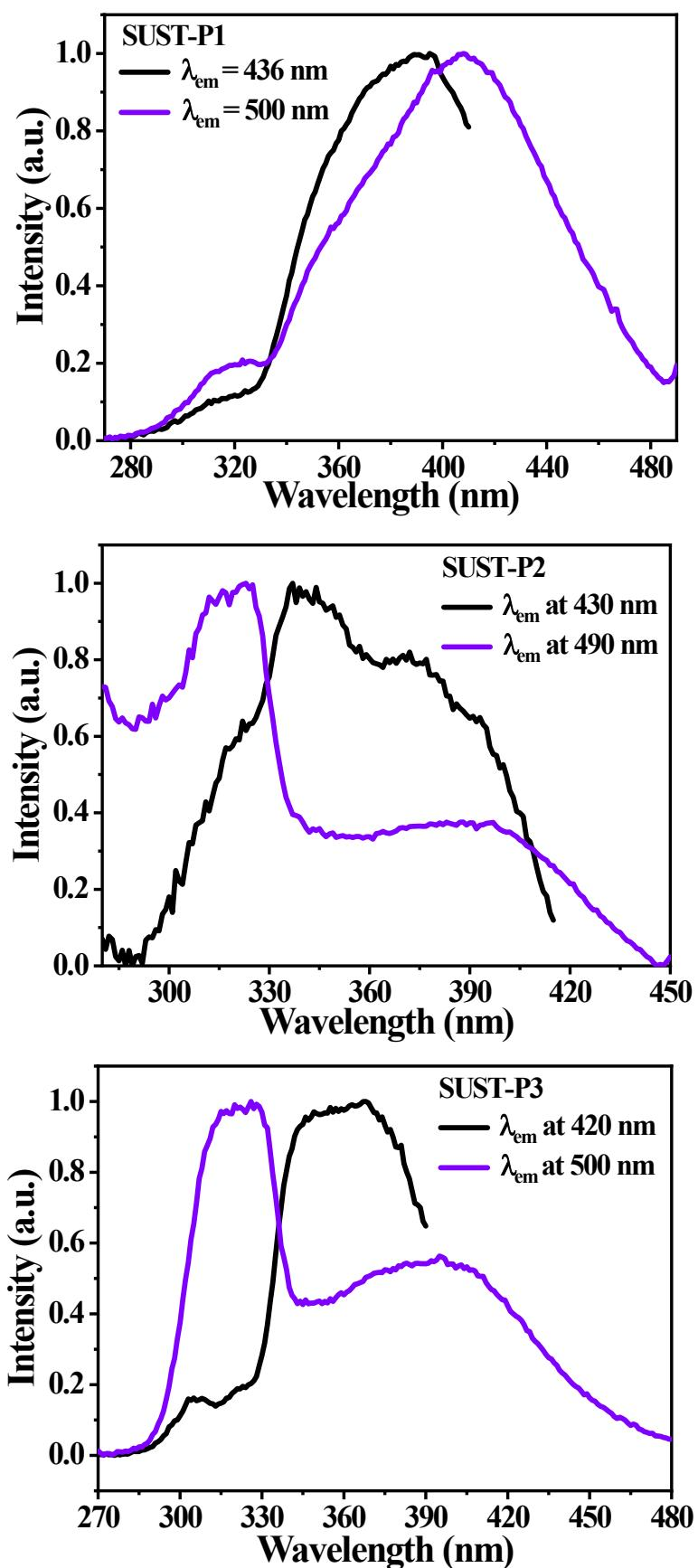
**Figure S19.** The excitation spectra of SUST-P1, SUST-P2 and SUST-P3 (room temperature, solid state).
