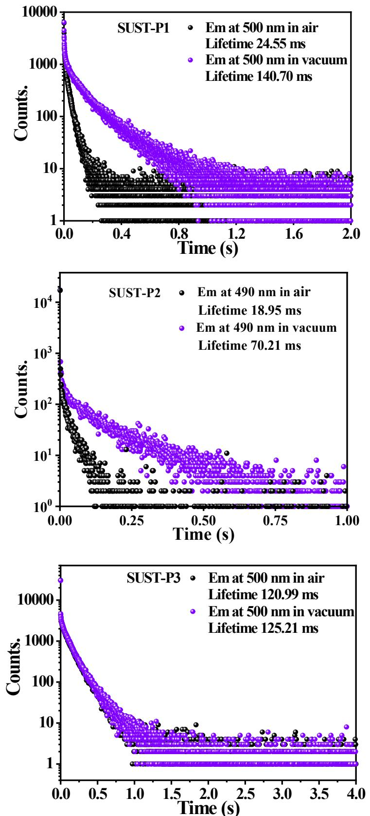
**Figure S18.** The decay curves of SUST-P1, SUST-P2 and SUST-P3 in air and vacuum at RT.
