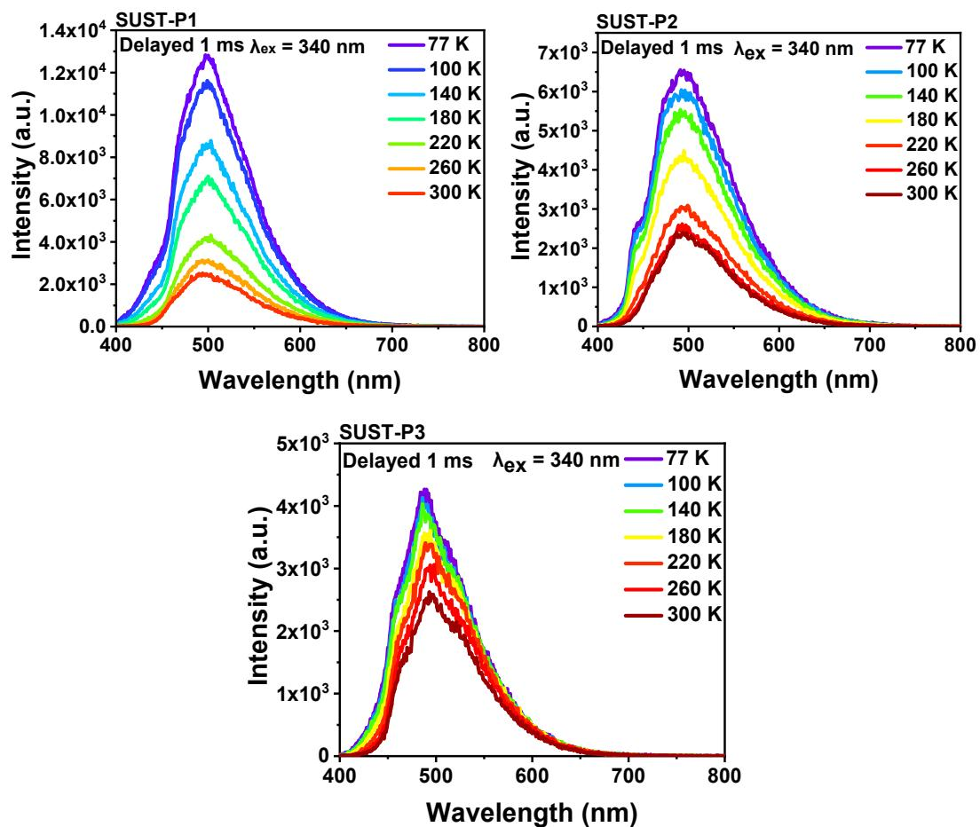
**Figure S15.** Temperature-dependent delayed spectra (delay 1 ms) of SUST-P1~P3 as the temperature dropped from 300 K to 77 K under 340 nm excitation.
