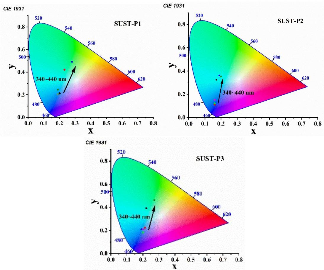
**Figure S21.** The CIE coordinates of SUST-P1, SUST-P2 and SUST-P3 corresponded to the excitation wavelength-dependent prompt emission spectra.
