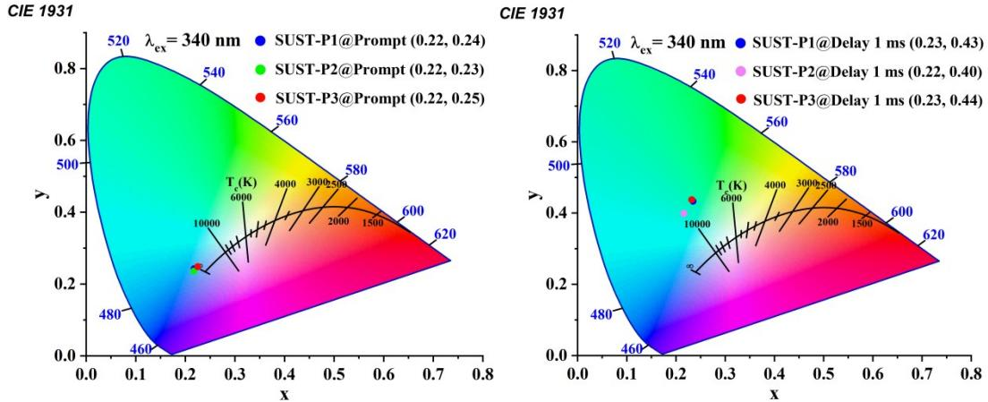
**Figure S12.** The CIE coordinates corresponding to the prompt and delayed (1 ms) photoluminescence spectra ( $\lambda_{\text{ex}} = 340$  nm).
