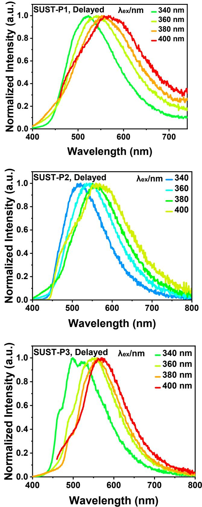
**Figure S23.** Excitation-dependent delayed emission spectra of SUST-P1, SUST-P2 and SUST-P3, respectively.
