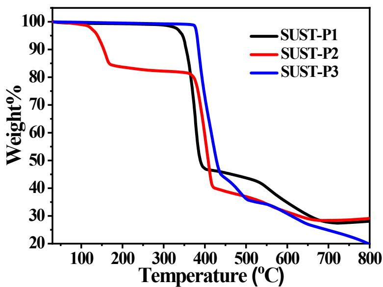
**Figure S3.** TGA curves of SUST-P1, SUST-P2 and SUST-P3.
