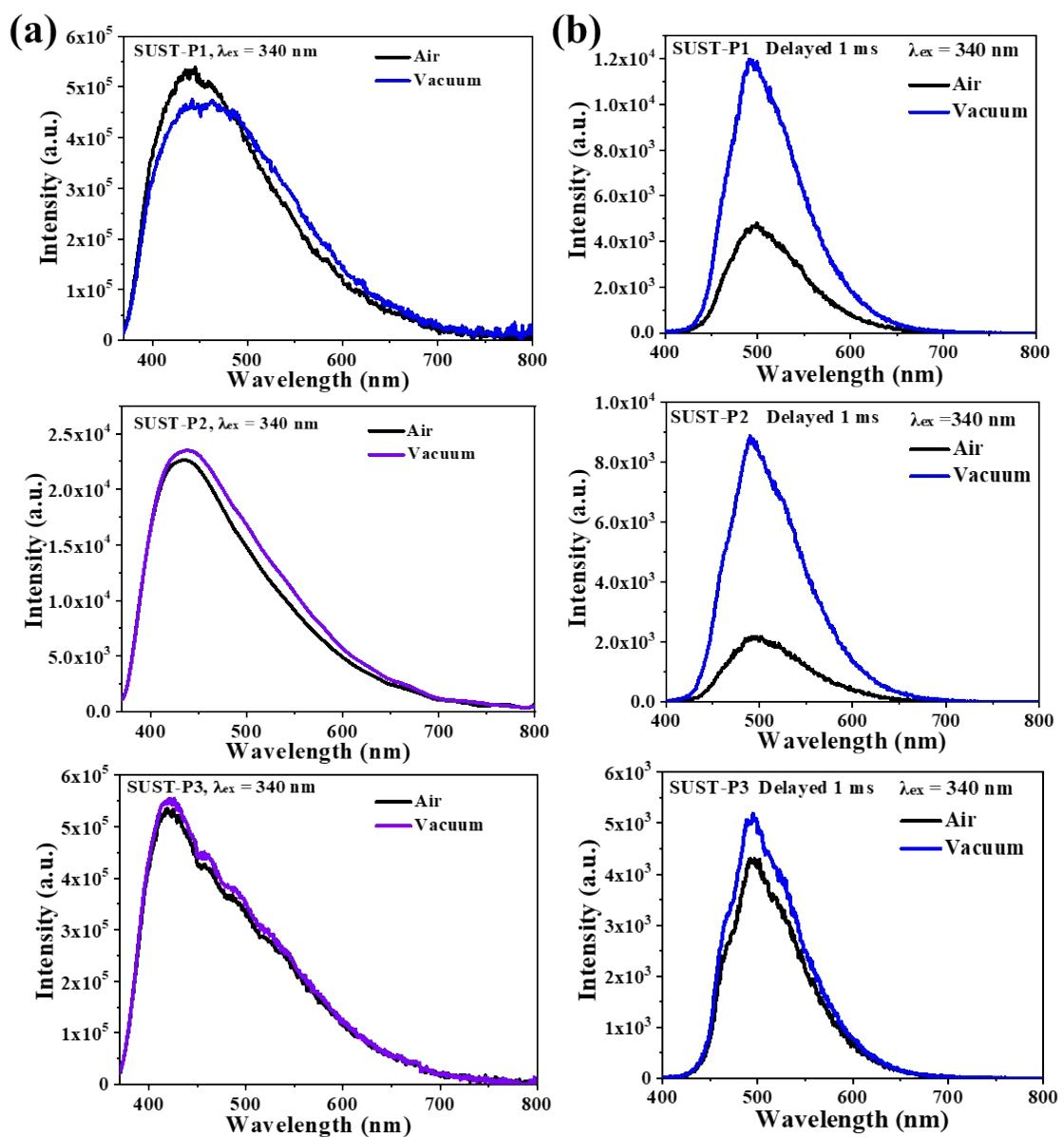
**Figure S17.** (a) The emission spectra of SUST-P1, SUST-P2 and SUST-P3 in air and vacuum at RT. (b) The delayed spectra of the three MOFs in air and vacuum at RT.
