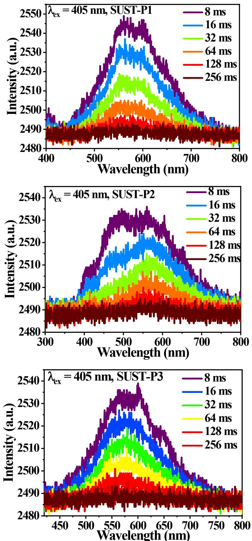
**Figure S22.** Long persistent luminescence (LPL) of SUST-P1, SUST-P2 and SUST-P3 upon the excitation at 405 nm.
