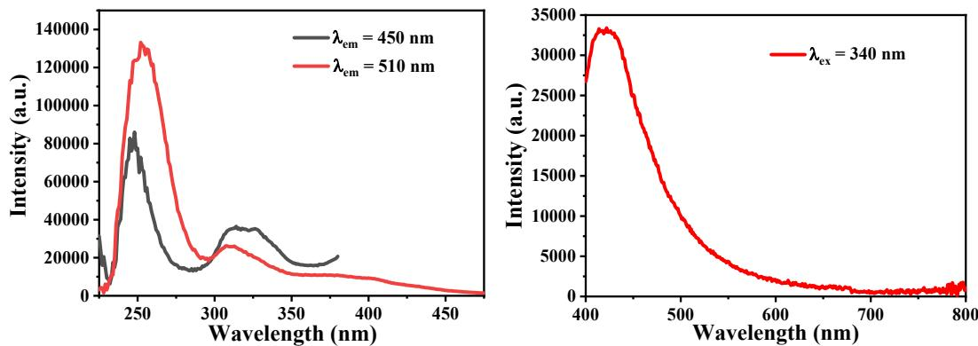
**Figure S9.** The excitation ( $\lambda_{\text{em}} = 450 \text{ nm}$  or  $510 \text{ nm}$ ) and emission ( $\lambda_{\text{ex}} = 340 \text{ nm}$ ) spectra of solid HL at room temperature.
