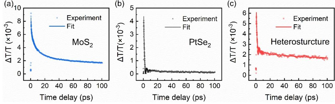
**Fig. S2** Experimental peak dynamics (symbols) and multi-exponential fitting results (lines). (a) A exciton bleaching signal at 1.86 eV probe energy from the bare MoS<sub>2</sub> sample. (b) Bleaching signal at 1.87 eV probe energy from the bare PtSe<sub>2</sub> sample. (c) A exciton bleaching signal at 1.87 eV probe energy from the heterostructure sample.
