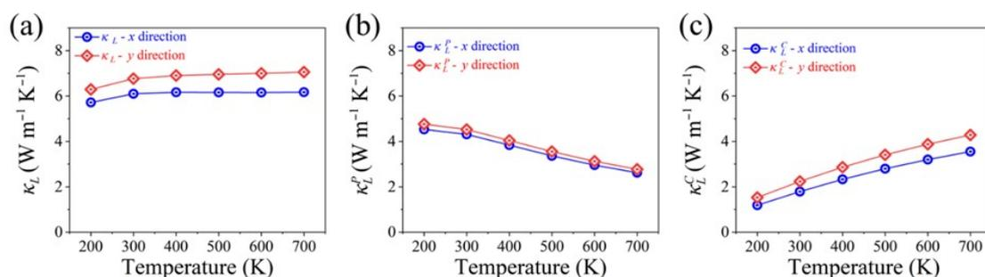
**Fig. S6.** (a) Total lattice thermal conductivity ( $\kappa_L$ ), (b) particle-like contribution ( $\kappa_L^P$ ), and (c) phonon coherence contribution ( $\kappa_L^C$ ) considering three-phonon scattering of the penta-PbN<sub>8</sub> sheet.
