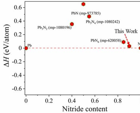
**Fig. S3.** The convex energy hull of the Pb<sub>x</sub>N<sub>1-x</sub> systems.
