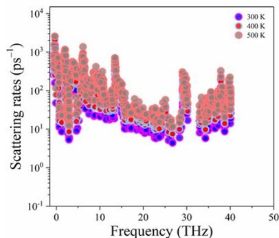
**Fig. S8** Scattering rates of the penta-PbN<sub>8</sub> sheet at temperatures of 300, 400, and 500 K.
