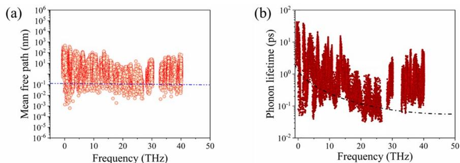
**Fig. S7.** Phonon means free path and phonon lifetime as a function of phonon frequency at 300 K for penta-PbN<sub>8</sub> sheet. The blue horizontal line is the average bond length (1.84 Å, Ioffe-Regel limits in space), and the black dashed curve is for the Ioffe-Regel limit ( $1/\omega$ ) in time.
