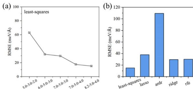
**Fig. S2** (a) Convergence test of the cutoff distances for the fitted interatomic force constant potential, and (b) comparison of different fitting methods.<sup>1</sup>
