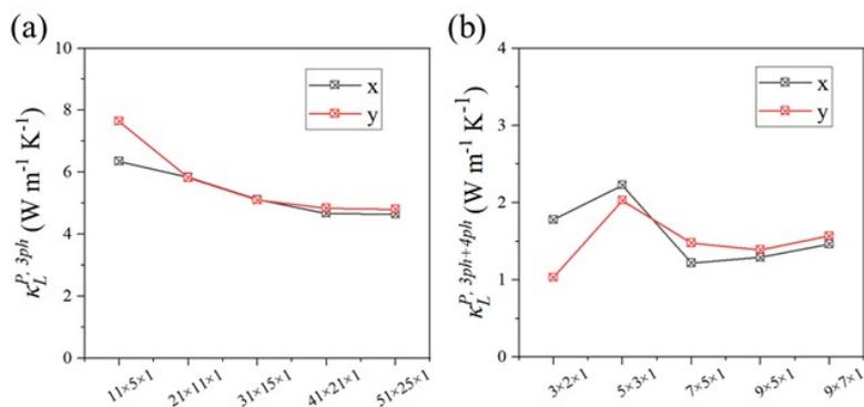
**Fig. S1** Convergence test of the calculations for (a) 3- and (b) 3+4 phonon scattering processes of the penta-PbN<sub>8</sub> sheet.
