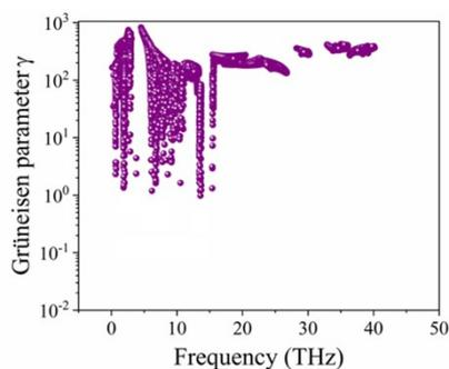
**Fig. S5.** Calculated Grüneisen parameter as a function of frequency for the penta-PbN<sub>8</sub> sheet.
