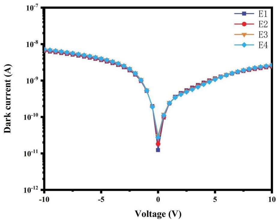
Figure S2. Dark current curves of the device at each electrode.
