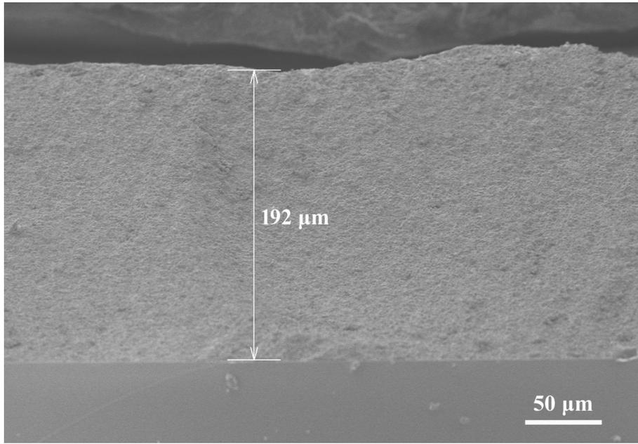
Figure S6. Cross-section of the comparison MAPbI<sub>3</sub> polycrystalline thick film
