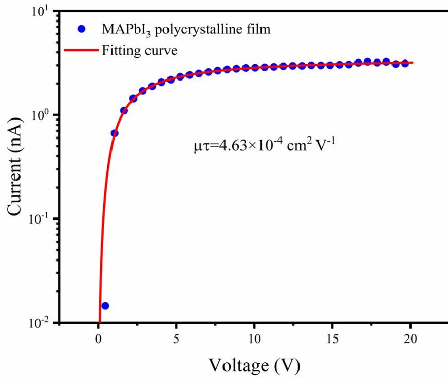
Figure S4. I-V characteristic curve of the comparison detector under X-ray irradiation.
