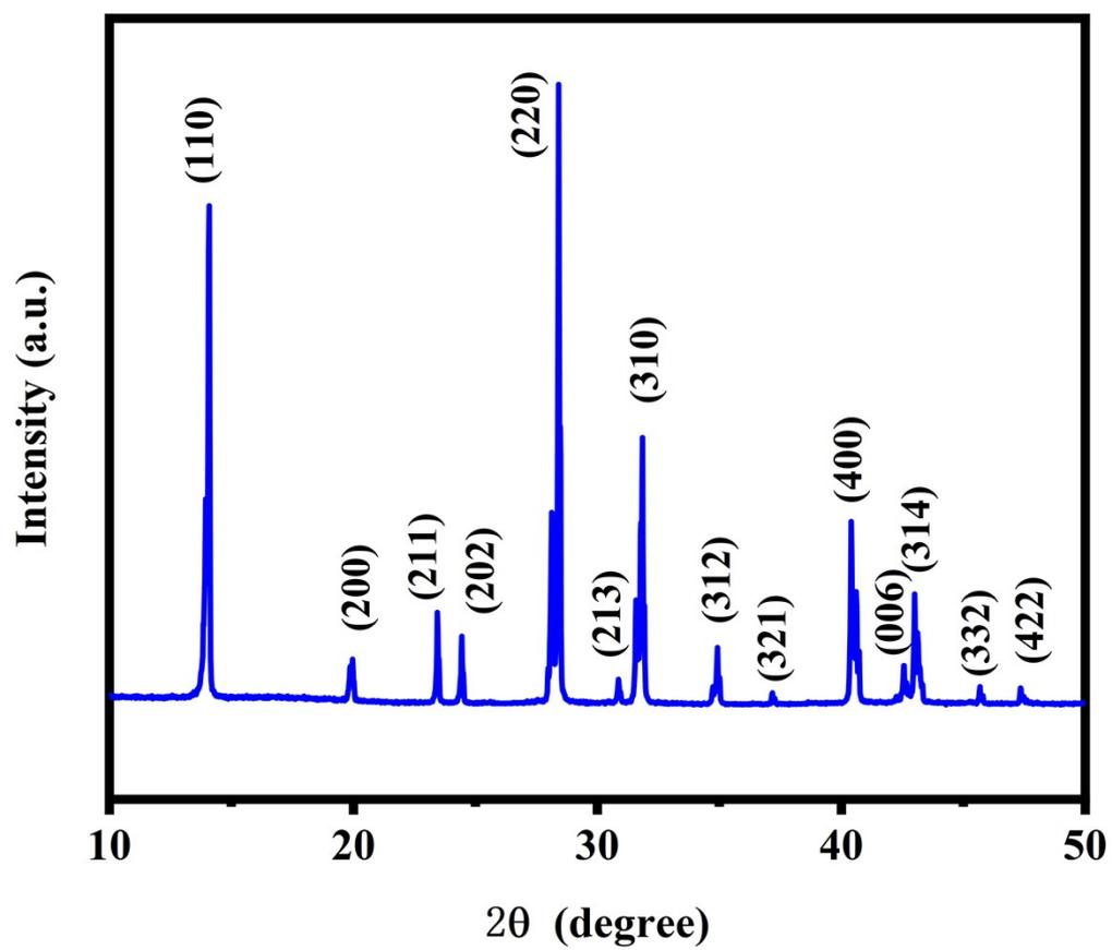
Figure S3. XRD patterns of MAPbI<sub>3</sub> thick film.
