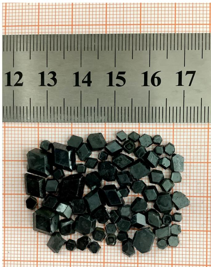
Figure S1. Photograph of the small-sized MAPbI<sub>3</sub> single crystals.
