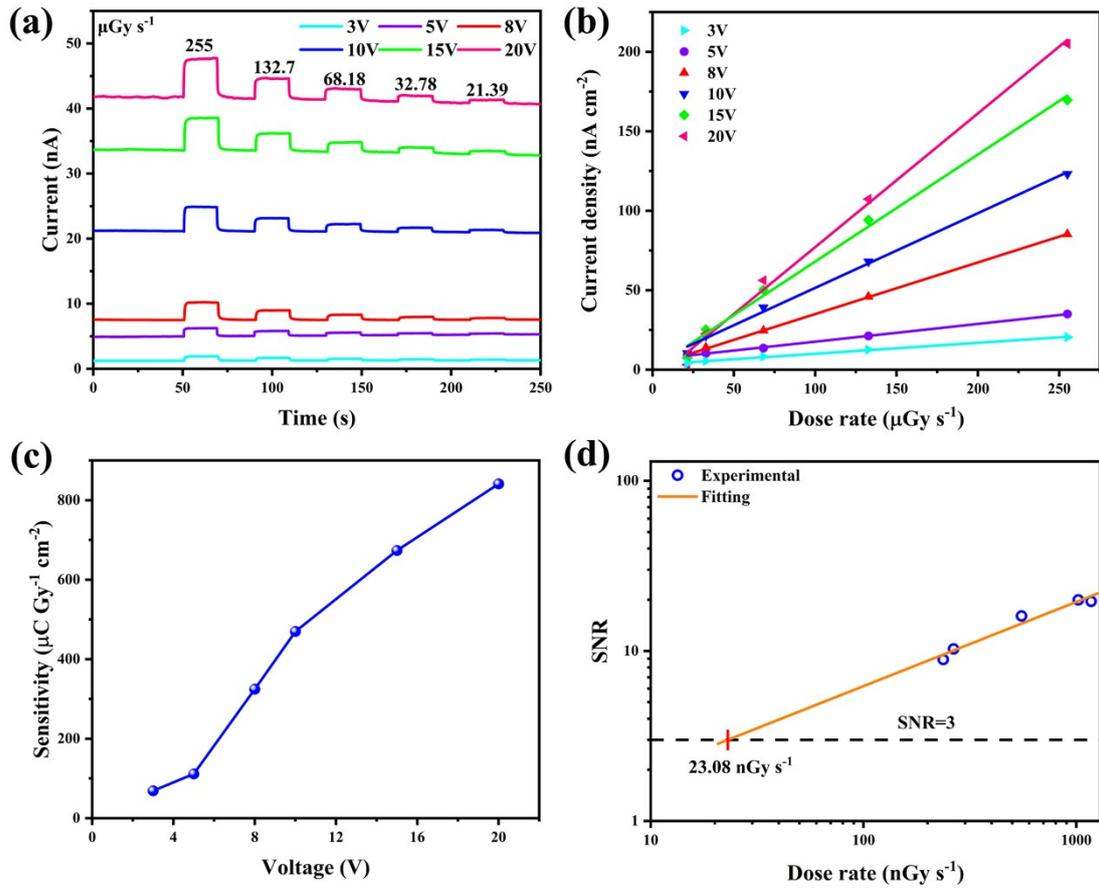
Figure S5. (a) X-ray response currents of the comparison detector were tested at different biases. (b) Photocurrent density of the comparison detector generated at different X-ray dose rates under various biases. (c) Sensitivity of the comparison detector generated at different X-ray dose rates under various biases. (d) The SNR of the comparison detector under different dose rates at 10 V bias.
