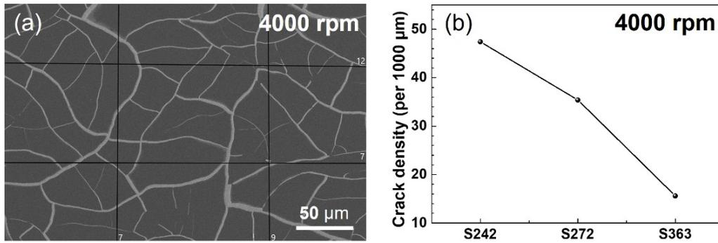
Fig. S2. Figuring calculations of (a) edge density of the metal-mesh structure and (b) crack density as a function of concentration at 4000 rpm.
