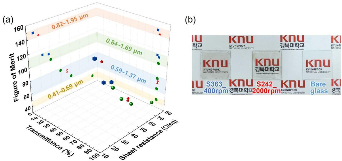
Fig. S5. (a) Figure of merit as a function of transmittance and sheet resistance in three dimensions based on Fig. 6, and (b) photograph images of samples for S363\_4000 rpm, S242\_2000 rpm, and bare glass substrate.
