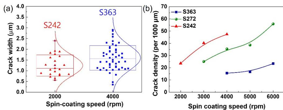
Fig. S4. (a) crack width distribution of S242\_2000rpm and S363\_4000rpm, (b) crack density of Ag micro-mesh electrodes.
