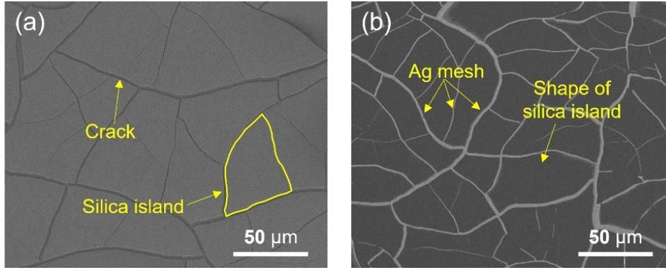
Fig. S1. SEM images of the (a) cracked template after drying the silica solution on the glass substrate and (b) Ag micro-mesh electrode grids after depositing the Ag thin film and lifting off the crack template. Shape of the Ag mesh corresponds to the cracks in the template along with the shape of the removed silica island.
