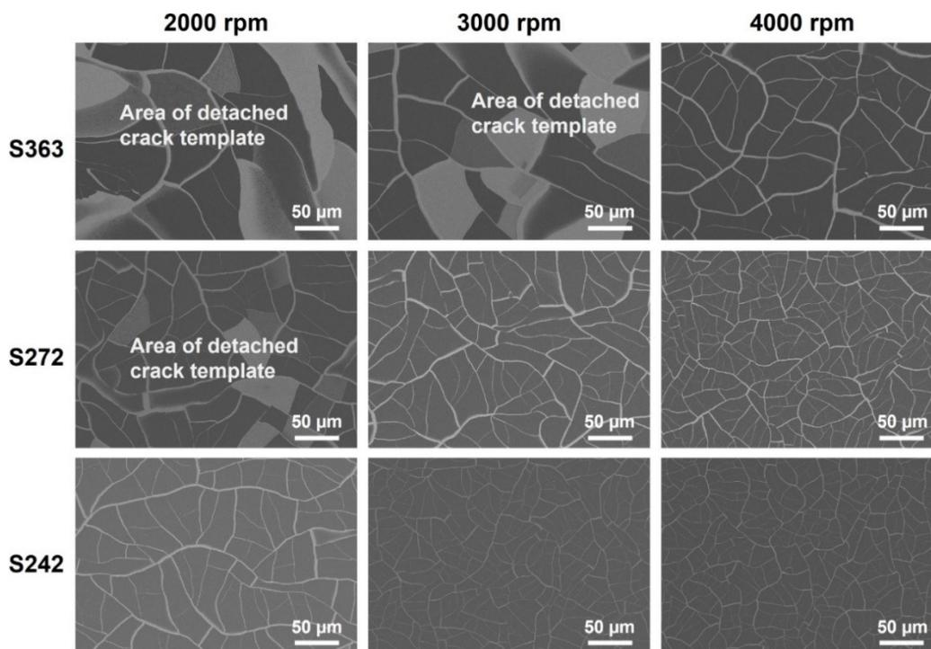
Fig. S3. SEM images of the S242, S272, and S363 samples fabricated at different spin-coating speeds.
