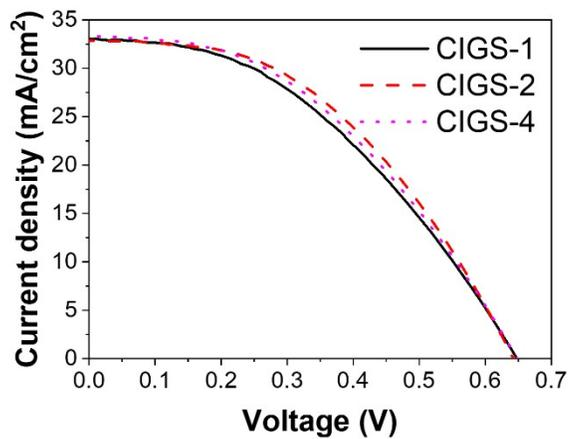
Fig. S6. Current density-voltage (J-V) curves of the CIGS solar cells with Ag micro-mesh electrodes.
