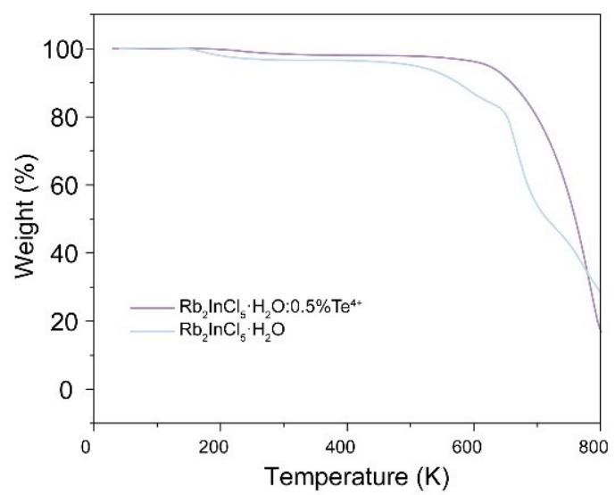
**Figure S4.** Thermogravimetric curves of  $\text{Rb}_2\text{InCl}_5 \cdot \text{H}_2\text{O}$  and  $\text{Rb}_2\text{InCl}_5 \cdot \text{H}_2\text{O}:0.5\%\text{Te}^{4+}$ .
