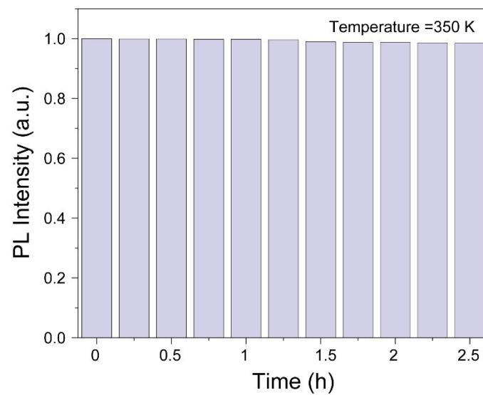
**Figure S10.** Fluorescent thermal stability at 350k.
