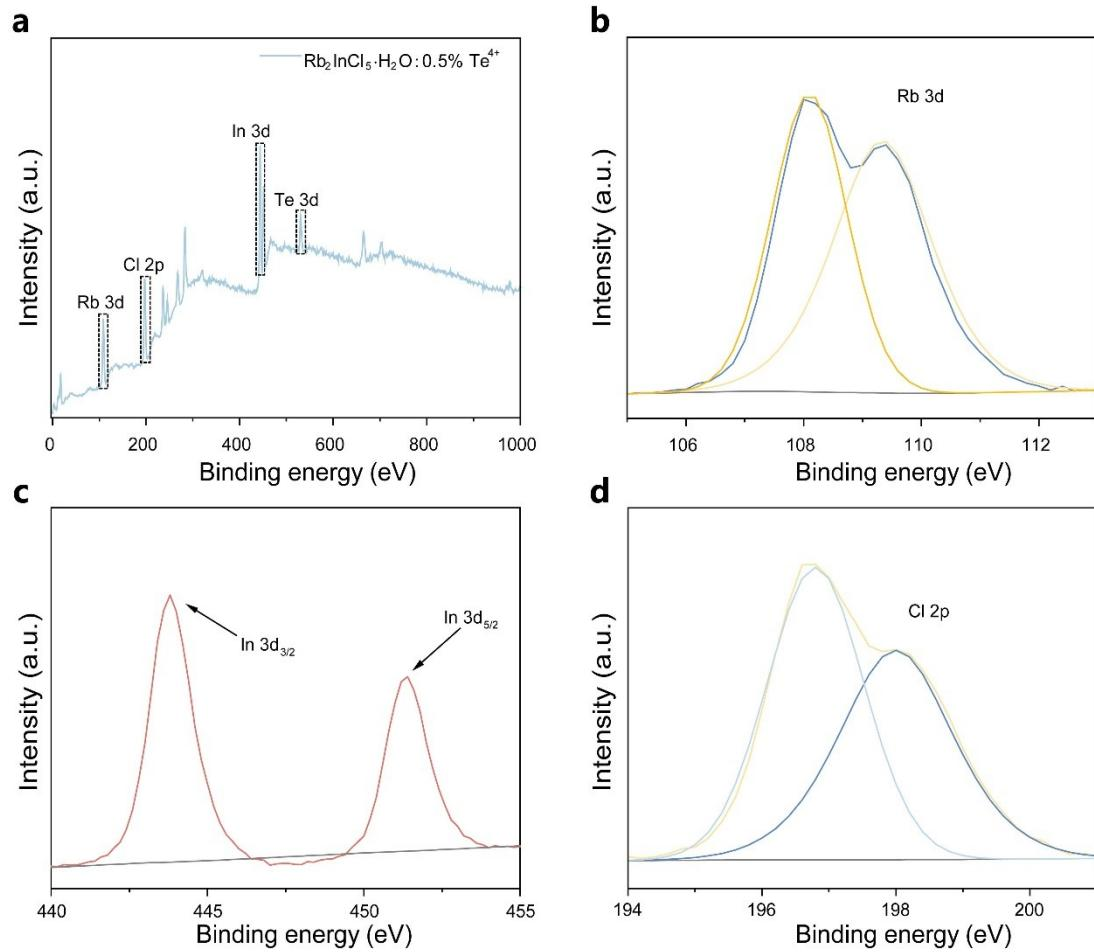
**Figure S2.** XPS survey spectrum of Rb<sub>2</sub>InCl<sub>5</sub>·H<sub>2</sub>O:0.5%Te<sup>4+</sup> a) The High-resolution XPS spectra of Rb<sub>2</sub>InCl<sub>5</sub>·H<sub>2</sub>O:0.5%Te<sup>4+</sup> corresponding to b) Rb 3d, c) In 3d and d) Cl 2P respectively.
