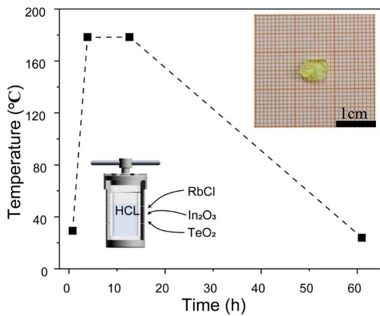
**Figure S1.** Showing the preparation procedure of  $\text{Rb}_2\text{InCl}_5 \cdot \text{H}_2\text{O}:\text{Te}^{4+}$  single crystal.
