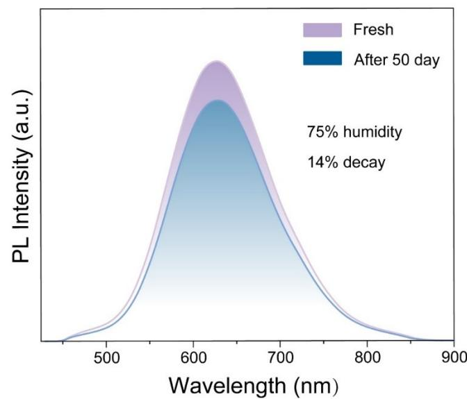
**Figure S9.** PL spectra of the  $\text{Rb}_2\text{InCl}_5 \cdot \text{H}_2\text{O}:0.5\%\text{Te}^{4+}$  single crystal before and after storage for 50 days in air ambient (75% humidity).
