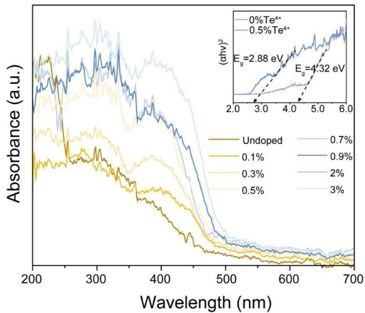
**Figure S5.** The spectra of  $\text{Rb}_2\text{InCl}_5 \cdot \text{H}_2\text{O}:x\text{Te}^{4+}$  ( $x=0.1\text{-}3\%$ ) and Tauc plots of  $\text{Rb}_2\text{InCl}_5 \cdot \text{H}_2\text{O}$  and  $\text{Rb}_2\text{InCl}_5 \cdot \text{H}_2\text{O}:0.5\%\text{Te}^{4+}$
