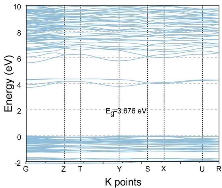
**Figure S6.** Calculated band structures for a  $\text{Rb}_2\text{InCl}_5 \cdot \text{H}_2\text{O}$ .
