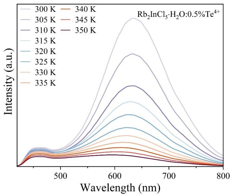
**Figure S8.** Temperature-dependent PL spectra of  $\text{Rb}_2\text{InCl}_5 \cdot \text{H}_2\text{O}:0.5\%\text{Te}^{4+}$ .
