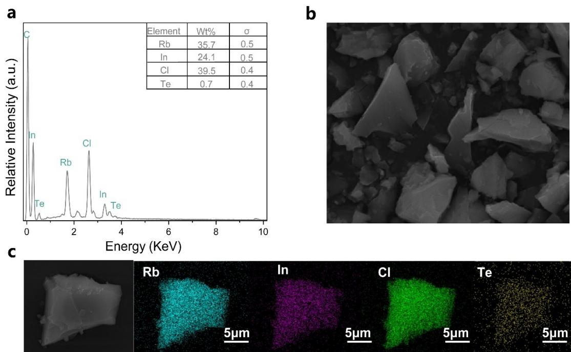
**Figure S3.** a) Energy disperse spectrum of  $\text{Rb}_2\text{InCl}_5 \cdot \text{H}_2\text{O}:0.5\%\text{Te}^{4+}$ . b) and c) SEM and EDS-mapping of selected area for  $\text{Rb}_2\text{InCl}_5 \cdot \text{H}_2\text{O}:0.5\%\text{Te}^{4+}$ .
