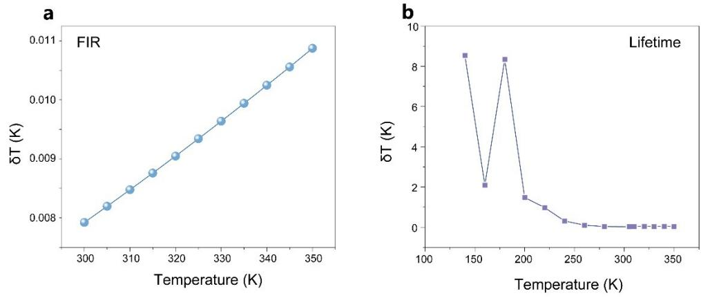
**Figure S11.** **a)** Temperature resolution of FIR mode in the temperature range from 300 K to 350 K. **b)** Temperature resolution of lifetime mode in the temperature range from 120 K to 350 K.
