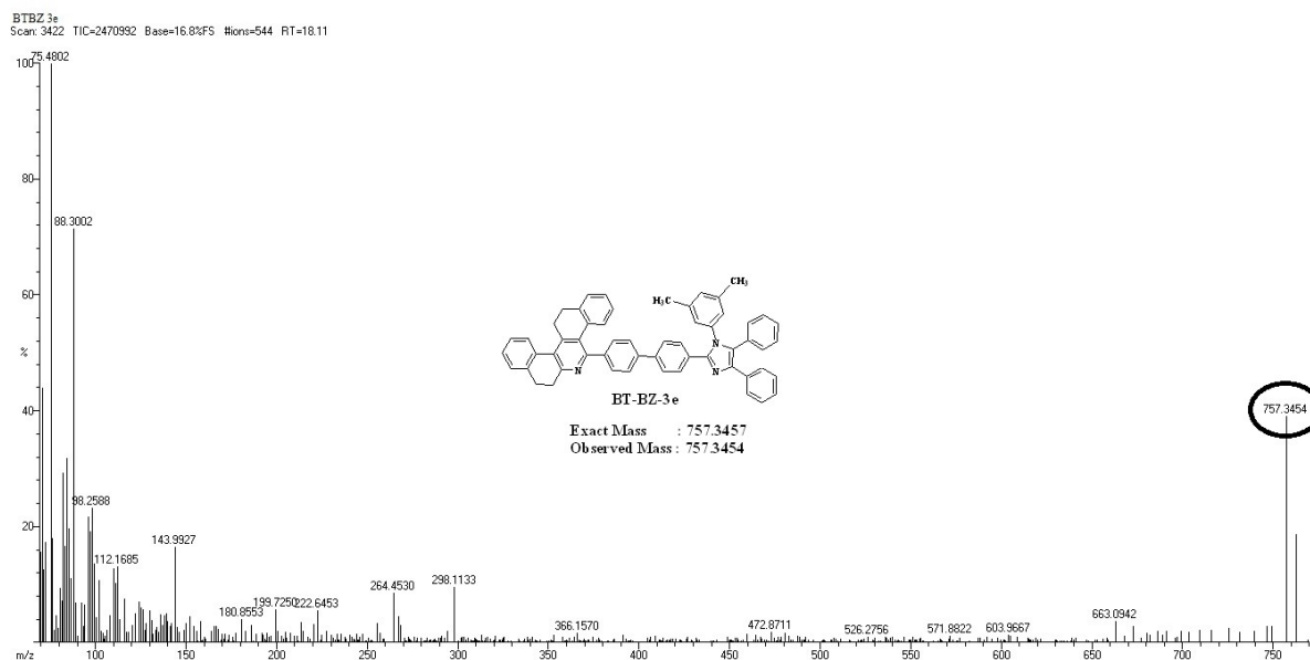
Fig. S3.5. HRMS Spectra of 5-(4'-(1-(3,5-dimethylphenyl)-4,5-diphenyl-1H-imidazol-2-yl)-[1,1'-biphenyl]-4-yl)-7,8,13,14-tetrahydrodibenzo[a,i]phenanthridine(3e)
