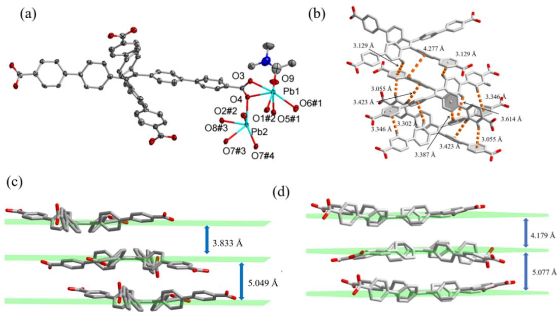
**Fig. S8.** (a) The coordination environments of  $\text{Pb}^{2+}$  cations in **1a** with the ellipsoids drawn at the 50% probability level. The hydrogen atoms are omitted for clarity. Symmetric code: #1  $-x+1, -y+1, -z+1$ ; #2  $-x, -y+1, -z+2$ ; #3  $-x+1, -y+2, -z+2$ ; #4  $x-1, y-1, z-1$ . (b) The  $\pi \dots \pi$  interactions between the  $\text{ETTC}^{4-}$  ligands in **1a**. The distances between adjacent  $\text{ETTC}^{4-}$  ligands in **1a** (c) and **1** (d).
