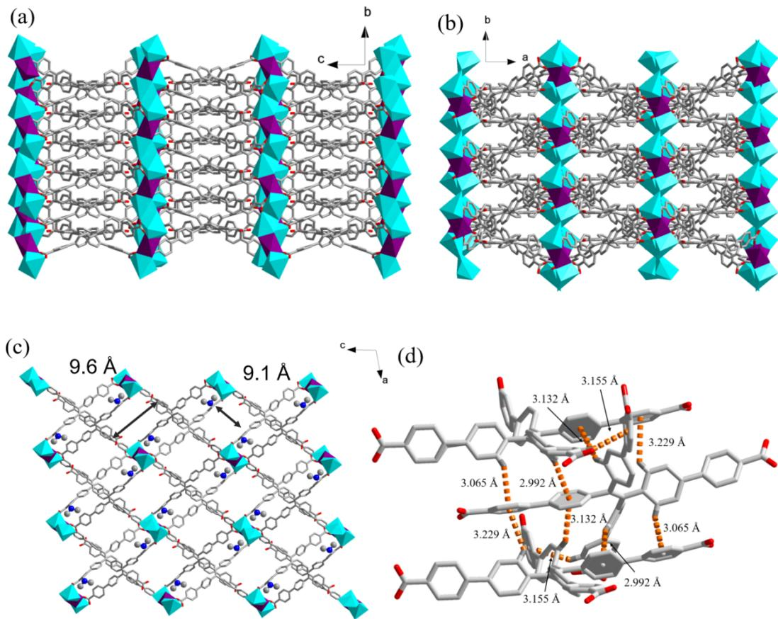
**Figure S2.** 3D coordination framework of complex **2** along *a*-axis (a) and *c*-axis (b). (c) The final structure of complex **2** with  $[(\text{CH}_3)_2\text{NH}_2]^+$  cations filled in the pores along *b*-axis. (d) The  $\pi \dots \pi$  interactions between the ETTC<sup>4-</sup> ligands in **2**.
