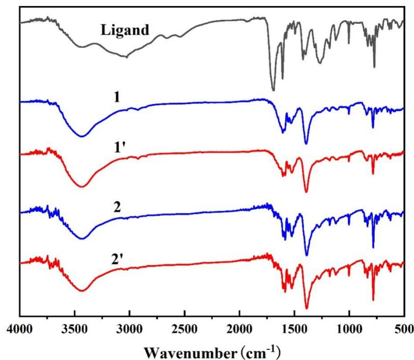
**Figure S4.** FT-IR spectra of organic ligand H<sub>4</sub>ETTC, MOFs **1** and **2**, MOFs **1'** and **2'** after recyclability tests.
