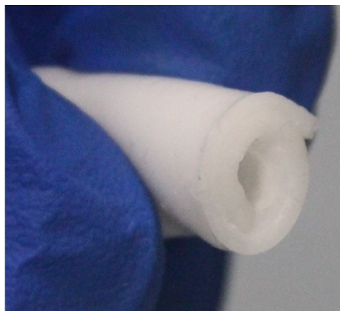
Figure S7. The flexible thin films composed by PDMS and LGO phosphor.
