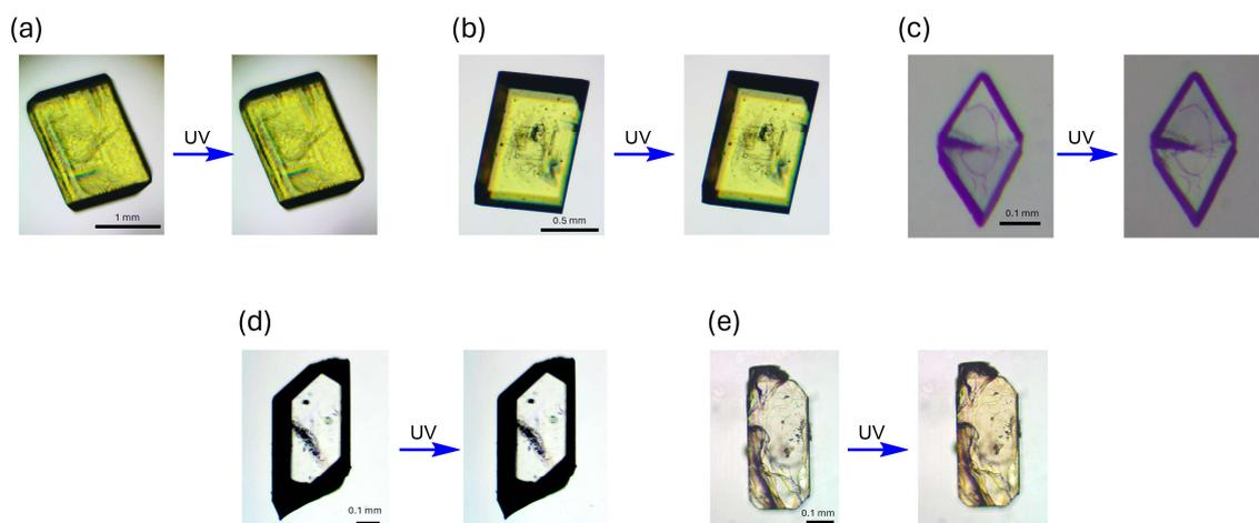
**Figure S11.** Optical microphotographs of crystal (a) **2o**, (b) **3o**, (c) **4o**, (d) **5o**, and (e) **6o-β** before and after upon irradiation with 365 nm light.
