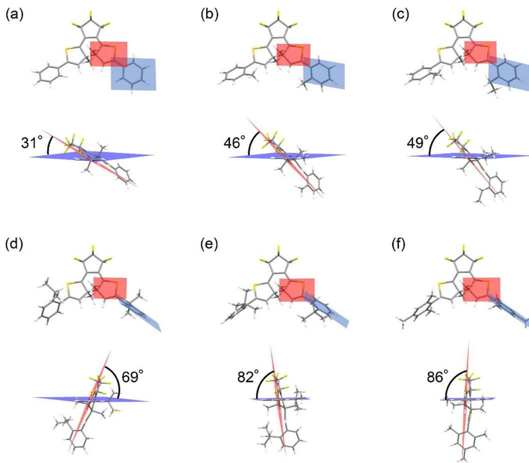
**Figure S2.** Optimized molecular structures and the dihedral angles in aryl groups of closed-ring isomers in solution by DFT calculation for (a) **1c**, (b) **2c**, (c) **3c**, (d) **4c**, (e) **5c**, and (f) **6c**.
