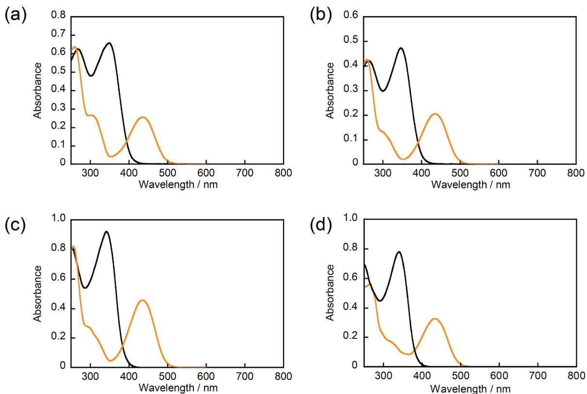
**Figure S3.** Absorption spectra of (a) **3** ( $3.8 \times 10^{-5} \text{ mol L}^{-1}$ ), (b) **4** ( $3.2 \times 10^{-5} \text{ mol L}^{-1}$ ), (c) **5** ( $6.2 \times 10^{-5} \text{ mol L}^{-1}$ ), and (d) **6** ( $4.9 \times 10^{-5} \text{ mol L}^{-1}$ ) in *n*-hexane: the open-ring isomer (black solid line) and the closed-ring isomer (orange solid line).
