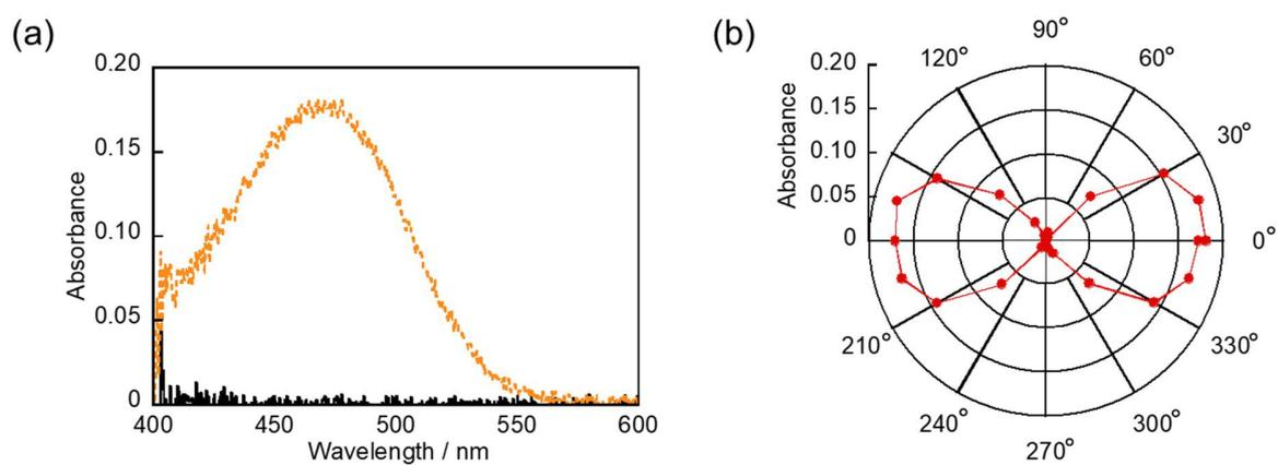
**Figure S16.** (a) Absorption spectra of crystal **7o** before and after UV irradiation, and (b) polar plots of the polarized absorption spectra of crystal **7o** at 470 nm on the (001) face.
