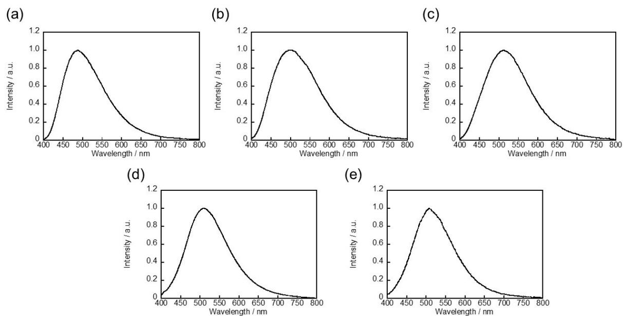
**Figure S5.** Fluorescence spectra of (a) **2**, (b) **3**, (c) **4**, (d) **5**, and (e) **6** in *n*-hexane upon excitation with 365 nm light.
