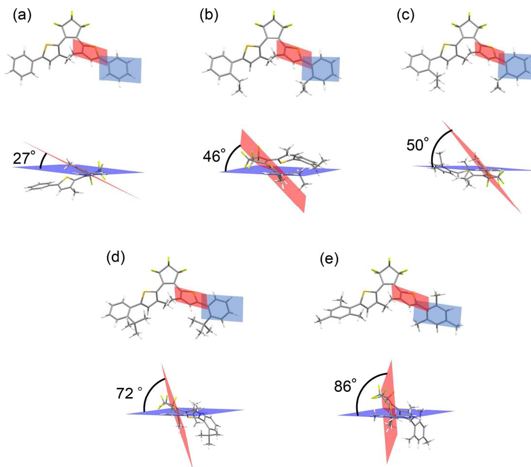
**Figure S1.** Optimized molecular structures and the dihedral angles in aryl groups of open-ring isomers in solution by DFT calculation for (a) **1o**, (b) **3o**, (c) **4o**, (d) **5o**, and (e) **6o**.
