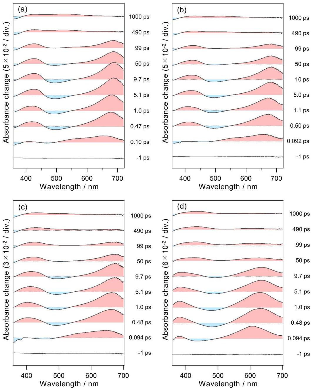
**Figure S8.** Transient absorption spectra of (a) **20**, (b) **30**, (c) **40** and (d) **50** in *n*-hexane excited with a femtosecond laser pulse at 350 nm.
