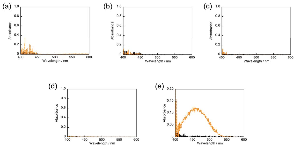
**Figure S12.** Absorption spectra of crystal (a) **2o**, (b) **3o**, (c) **4o**, (d) **5o**, and (e) **6o-β** before (black line) and after (orange line) upon irradiation with 365 nm light.
