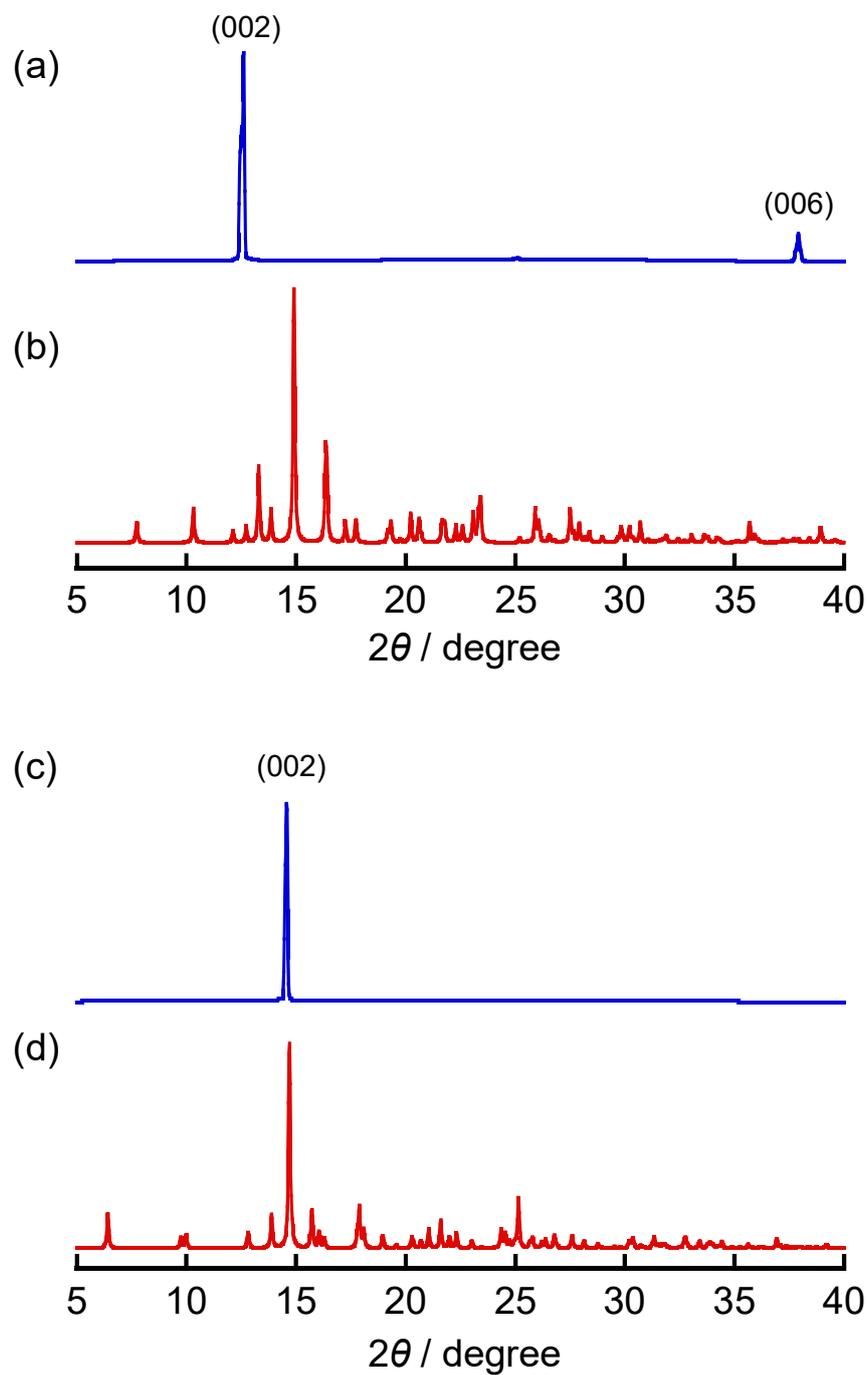
**Figure S14.** PXRD patterns of crystal (a) **60- $\alpha$**  and (c) **60- $\beta$** . The patterns calculated from single crystal X-ray crystallographic data of (b) **60- $\alpha$**  and (d) **60- $\beta$** .
