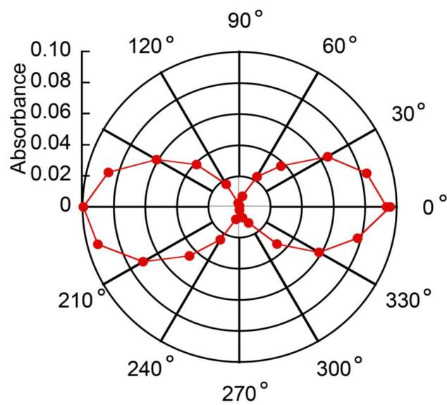
**Figure S13.** Polar plots of the polarized absorption spectra of crystal **60-β** at 455 nm on the (001) face.
