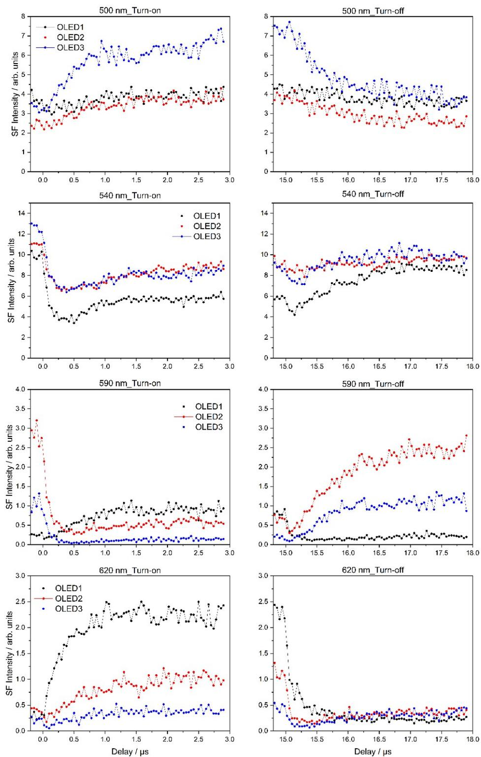
**Figure S4.** Transient ESFG (rise and fall) intensities of three different OLED devices at four visible wavelengths upon the application of the square wave pulse bias.
