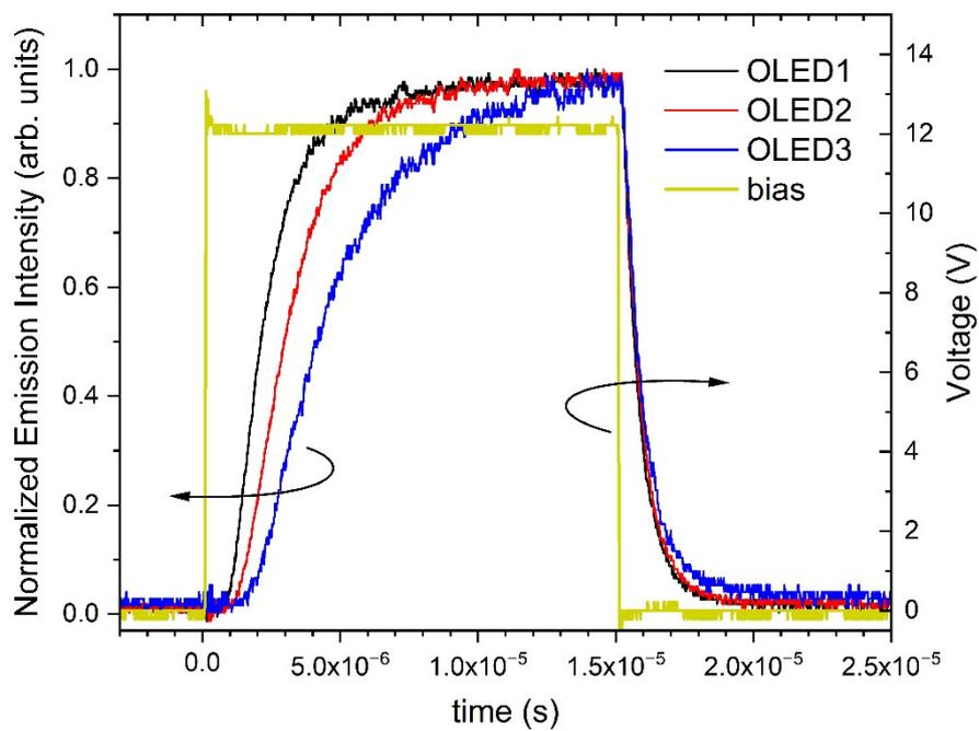
**Figure S5.** Transient EL emission of three OLED devices when square wave pulse voltage is applied.
