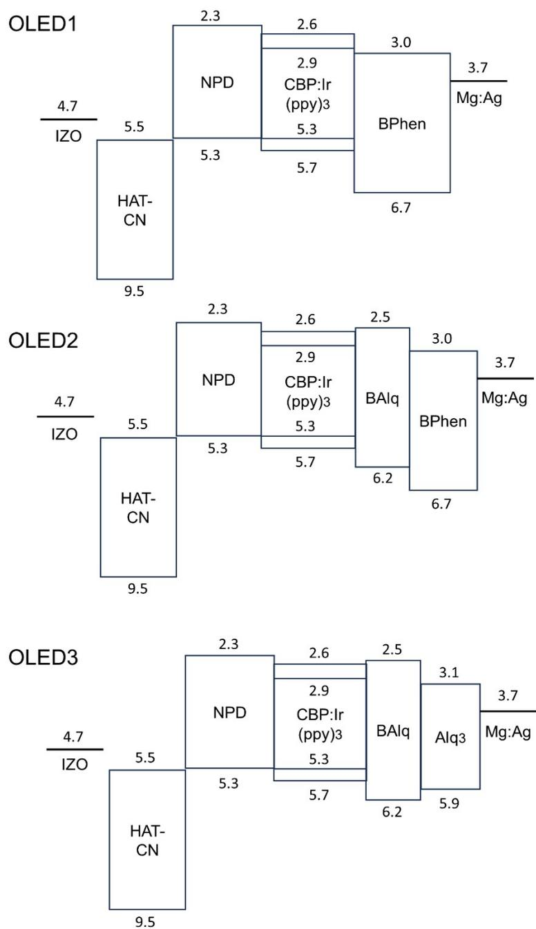
**Figure S1.** The energy diagrams with respect to the vacuum level of the organic materials used in each OLED device. HOMO/LUMO energies of each material and the work functions of IZO and Mg:Ag in **Fig. S1** are cited from below references.
