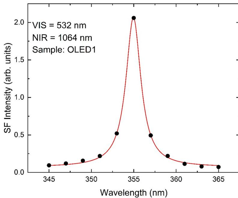
**Figure S2.** Spectral bandwidth of the output light when 1064 and 532 nm lights are irradiated to OLED1 at 62° and 70°, respectively.
