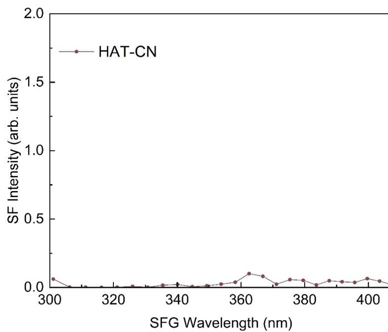
**Figure S3.** ESFG spectrum of the 100 nm thick HAT-CN film on CaF<sub>2</sub>. Polarization combination is ppp.
