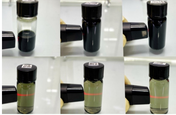
Fig. S1. Tyndall effect diagram of \text{Ti}_3\text{C}_2\text{T}_x dispersions.
