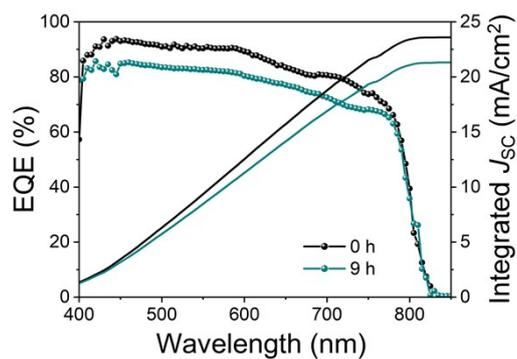
**Fig. S1** External quantum efficiency (EQE) curves and integrated current densities of PSCs fabricated from perovskite precursor solution aged at 0 h and 9 h.
