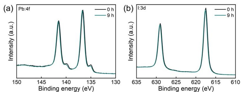
**Fig. S4** XPS spectra of perovskite films prepared from the precursor solution aged for 0 h and 9 h.
