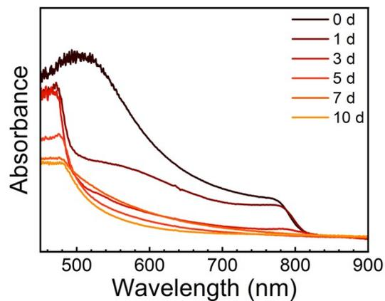
**Fig. S7** UV-visible spectra of films prepared from the precursor solution aged in different times.
