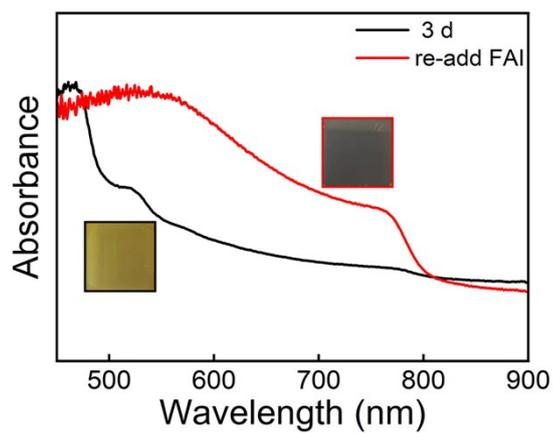
**Fig. S8** UV-visible spectra of the films prepared from the solution after 3 d of aging using the M\_D strategy and the solution of re-add 0.5 M FAI.
