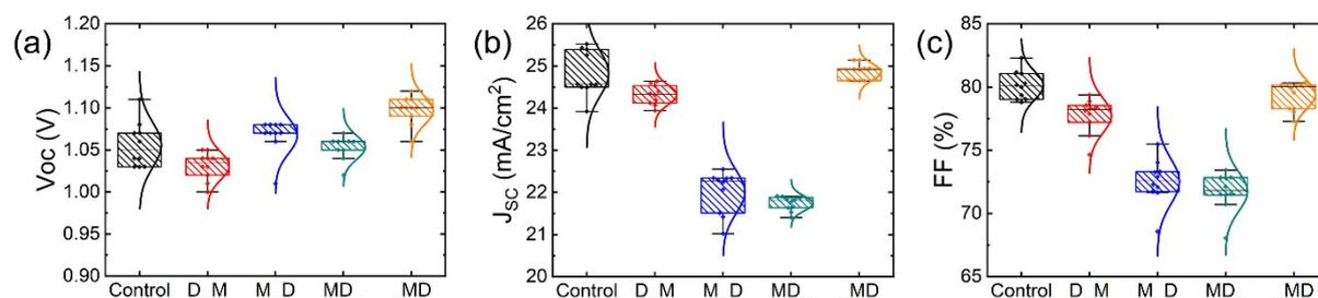
**Fig. S10** Statistical photovoltaic parameters of (a) open-circuit voltage ( $V_{oc}$ ), (b) short-circuit photocurrent density ( $J_{sc}$ ), (c) fill factor (FF) of perovskite solar cells aged in different sequential addition strategies.
