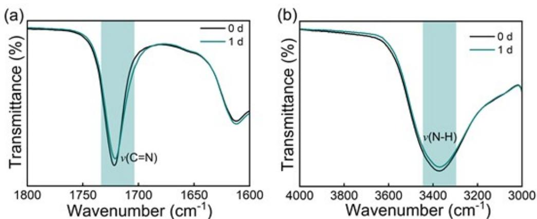
**Fig. S6** (a, b) Fourier transform infrared spectroscopy of precursor solution aged for 0 d and 1 d.
