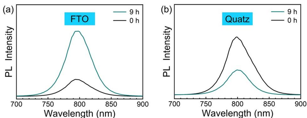
**Fig. S5** SSPL of perovskite films prepared from the precursor solution aged for 0 h and 9 h on (a) FTO and (b) quartz substrates.
