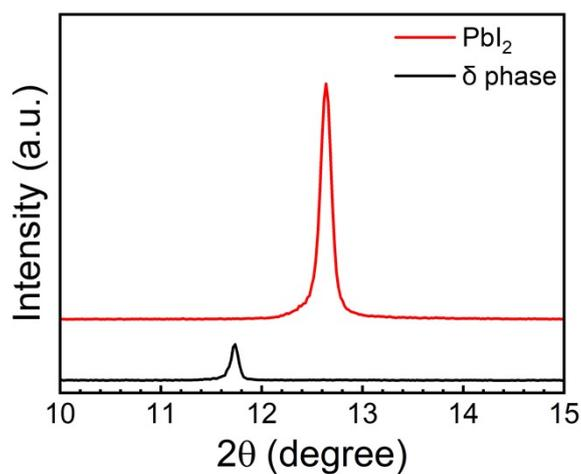
**Fig. S3** X-ray diffraction (XRD) patterns of  $\text{PbI}_2$  and  $\delta$ -phase perovskite.
