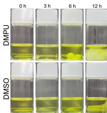
**Fig. S9** Images of the solute component extracted from the perovskite precursor solution with the addition of a combination of DMPU and RACl by using EA antisolvent.
