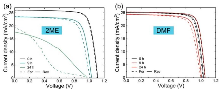
**Fig. S2**  $J$ - $V$  curves of PSCs prepared using 2-ME (a) and DMF (b) precursor solution aged for 0 h, 9 h and 24 h.
