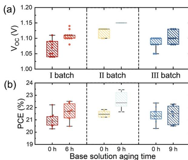
**Fig. S11** Changes of (a)  $V_{oc}$  and (b) PCE in PSCs prepared from precursor solutions with different base solution aging time.
