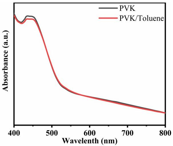
**Fig. S5** UV-vis absorption spectra of perovskite films without and with toluene modification.
