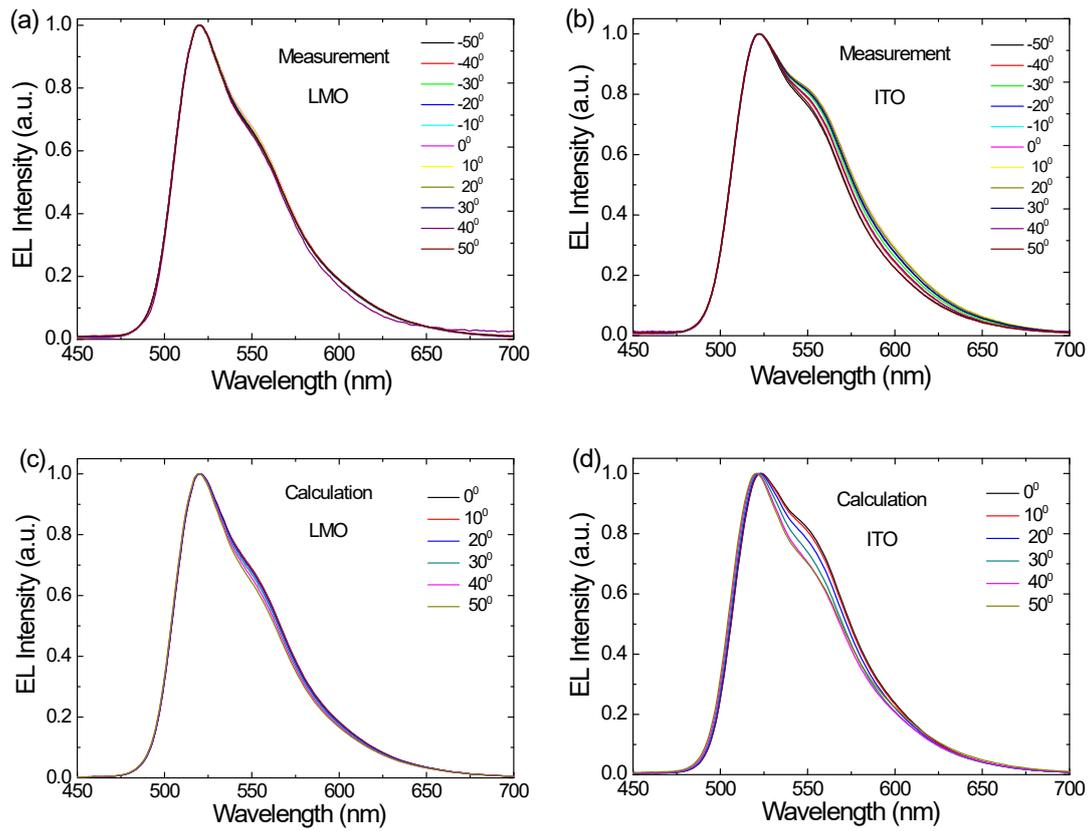
**Fig. S2.** Measurement emission spectra at various angles from an OLED with (a) LMO electrode, (b) ITO electrode. Calculated spectral radiance for OLED with (c) LMO electrode, (d) ITO electrode.
