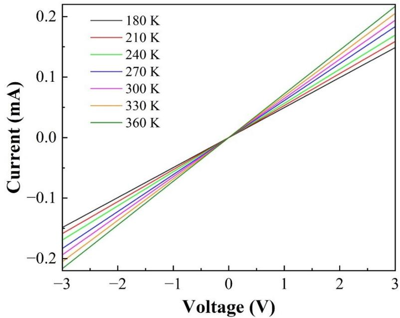
**Fig. S7.** Current–Voltage characteristics range from 180 K to 360 K of Glass/ Al finger electrodes (100 nm)/MoO<sub>3</sub> (2 nm)/Al (2 nm)/MoO<sub>3</sub> (5 nm)/NPB (100 nm).
