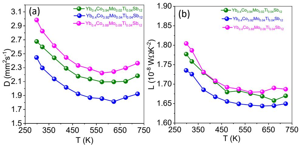
Fig. S8 (a) Thermal diffusivity as a function of temperature (b) Variation of Lorenz number with temperature
