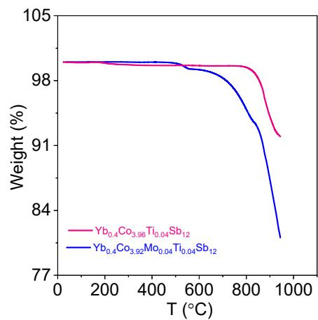
Fig. S2 Differential scanning calorimetry (DSC) measurement on  $\text{Yb}_{0.4}\text{Co}_{3.96}\text{Ti}_{0.04}\text{Sb}_{12}$  and  $\text{Yb}_{0.4}\text{Co}_{3.92}\text{Mo}_{0.04}\text{Ti}_{0.04}\text{Sb}_{12}$  in the temperature range 30 °C to 950 °C.
