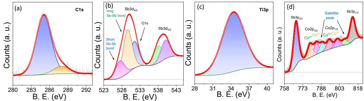
Fig. S3 XPS spectra of (a) C1s, (b) Sb3d (c) Ti3p, and (d) Co2p, Sb3p for energy levels of  $\text{Yb}_{0.4}\text{Co}_{3.88}\text{Mo}_{0.08}\text{Ti}_{0.04}\text{Sb}_{12}$ .
