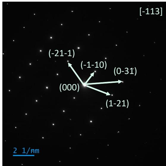
Fig. S9 BCC SAED single orientation pattern captured from single grain
