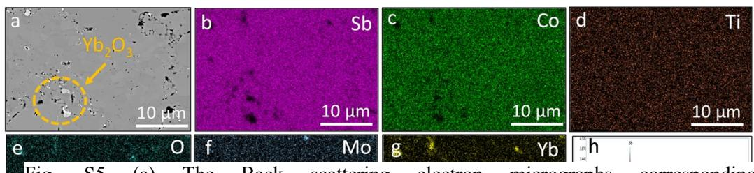
Fig. S5 (a) The Back scattering electron micrographs corresponding  $\text{Yb}_{0.4}\text{Co}_{3.88}\text{Mo}_{0.08}\text{Ti}_{0.04}\text{Sb}_{12}$ . (b), (c), (d), (e), (f) and (g) denotes the elemental mapping of O, Ti, Mo, Yb, Sb, and Co elements respectively. (h) EDS spectra of  $\text{Yb}_{0.4}\text{Co}_{3.92}\text{Mo}_{0.04}\text{Ti}_{0.04}\text{Sb}_{12}$
