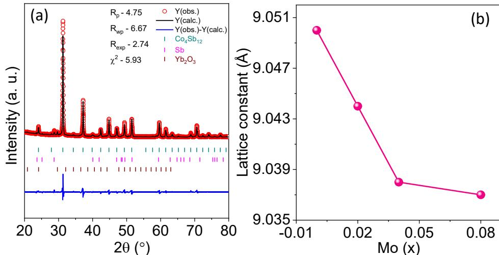
Fig. S1 (a) The Rietveld refinement of  $\text{Yb}_{0.4}\text{Co}_{3.88}\text{Mo}_{0.08}\text{Ti}_{0.04}\text{Sb}_{12}$  composition (b)
