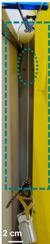
**Fig. S17:** SHP 2.0 stretching from a length at rest of 1.2 cm up to a length of 20 cm upon 20 mg weight loading. The circle area indicates the cut-healed area after 12 hours of self-healing process. Further, our fiber, following a 12-hours self-healing process, were attached to a 20 mg weight and stretched up to 1200 % elongating from 1.2 to 20 cm, highlighting remarkable strength.
