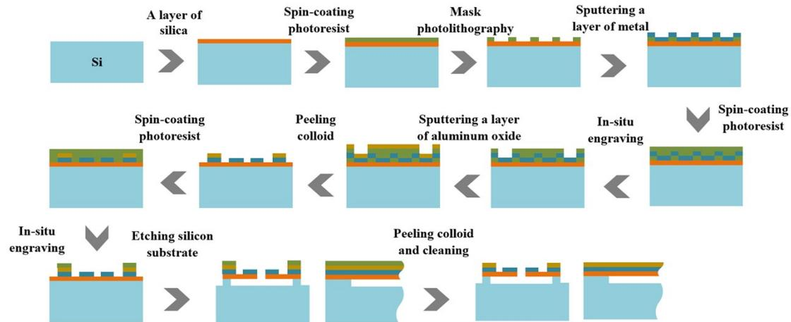
Figure S1. Fabrication process of suspended microelectrodes.
