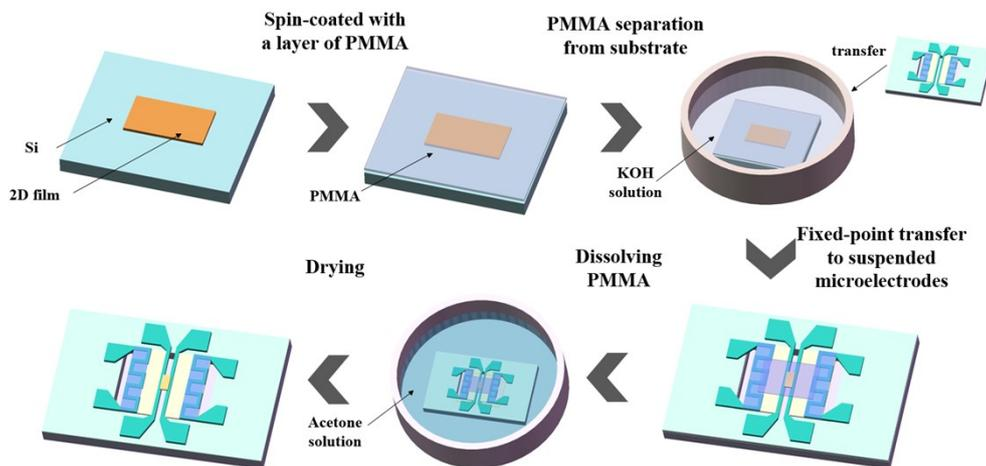
Figure S2. Transfer process with PMMA method.
