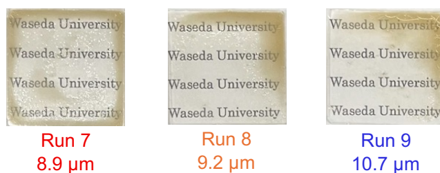
Fig. S30. Thin films (including their thickness) of CP3 on glass substrates.
