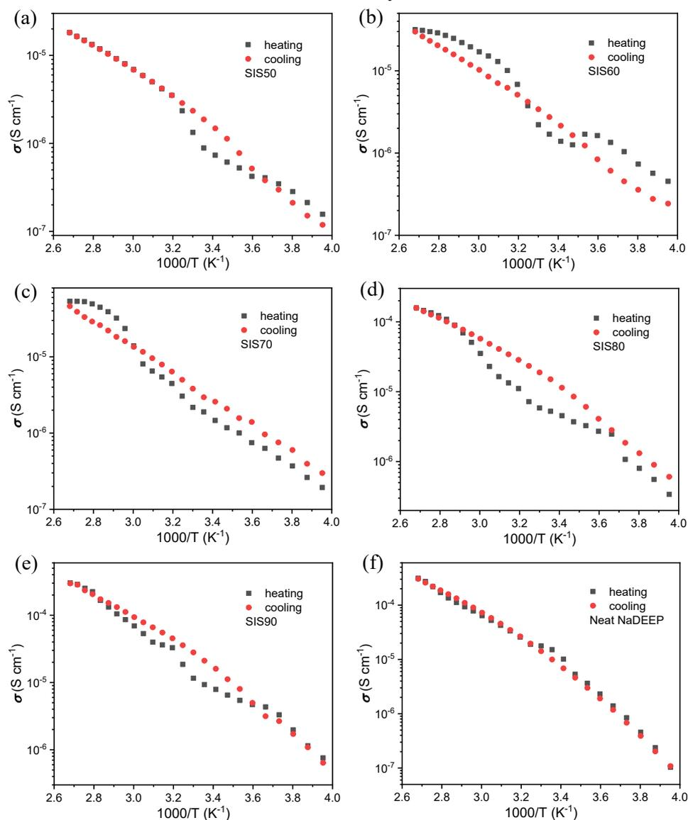
**Figure S2.** Ionic conductivities for (a-e) the SISXX electrolytes and (f) NaDEEP as a function of temperature.
