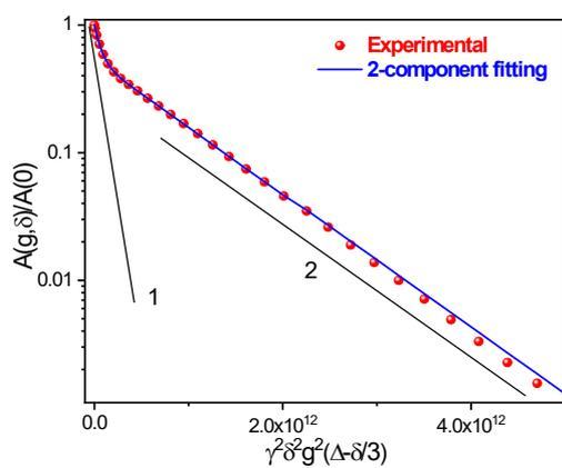
**Figure S8.** Experimental  $^1\text{H}$  diffusion decay at 303 K and a two-component fitting for the SIS50 electrolyte.
