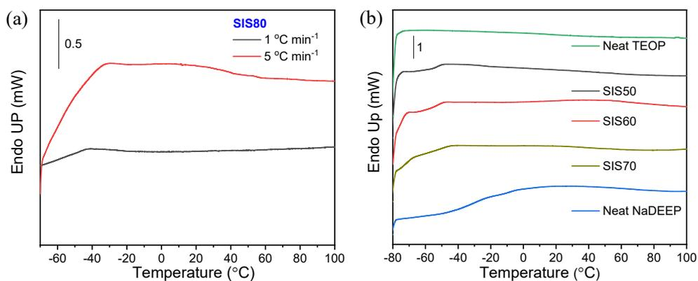
**Figure S1.** DSC traces of (a) SIS80 from -80 to 100 °C at 1 and 5 °C·min<sup>-1</sup>, and (b) the NaDEEP salt, the TEOP solvent, and selected SISXX electrolytes from -80 to 100 °C at 5 °C·min<sup>-1</sup>.
