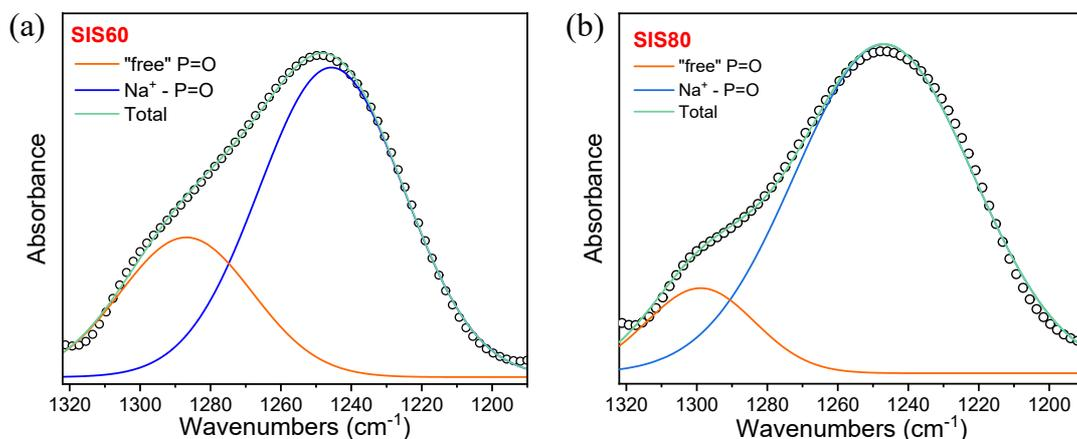
**Figure S5.** Deconvolution the P=O stretching vibrational mode for the SIS60 and SIS80 electrolytes.
