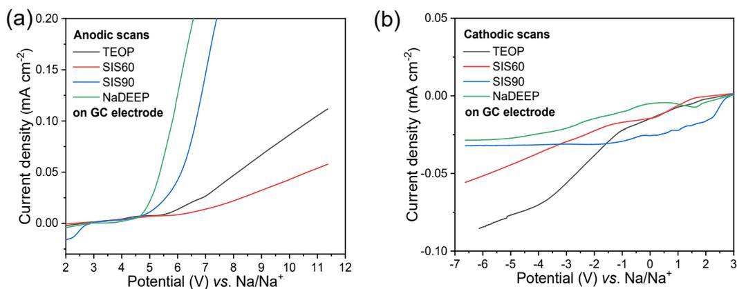
**Figure S4.** Anodic (a) and cathodic (d) LSV scans of TEOP solvent, SIS60, SIS90 and NaDEEP salt using a GC WE.
