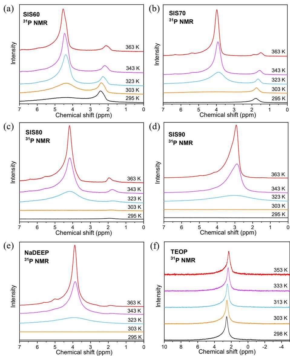
**Figure S6.**  $^{31}\text{P}$  NMR spectra of (e) the NaDEEP salt, (f) the TEOP solvent, and (a-d) the SISXX electrolytes.
