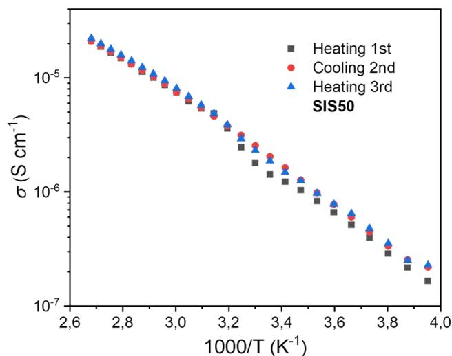
**Figure S3.** Ionic conductivities for the SIS50 electrolyte during heating-cooling-heating cycle.
