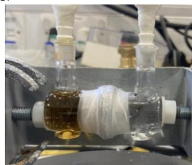
Figure S3: H-Cell set-up used to measure cross-over of negolyte.
