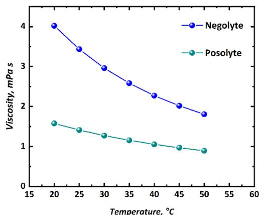
Figure S2: Viscosities of posolyte (0.25 M  $\text{Na}_4[\text{Fe}(\text{CN})_6]$ , 0.25 M  $\text{K}_4[\text{Fe}(\text{CN})_6]$ , 1.00 M NaCl) and negolyte (0.50 M  $\text{FeCl}_3$ , 1.00 M BIS-TRIS, 2.50 M NaOH) as a function of temperature.
