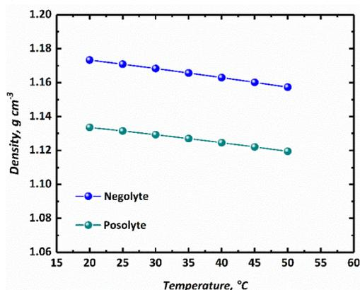
Figure S1: Densities of posolyte (0.25 M  $\text{Na}_4[\text{Fe}(\text{CN})_6]$ , 0.25 M  $\text{K}_4[\text{Fe}(\text{CN})_6]$ , 1.00 M NaCl) and negolyte (0.50 M  $\text{FeCl}_3$ , 1.00 M BIS-TRIS, 2.50 M NaOH) as a function of temperature.
