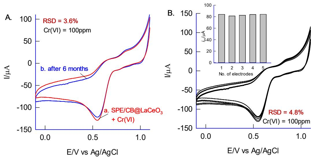
**Figure S8.** A) Reproducibility test of SPE/CB@LaCeO<sub>3</sub> before and after 6 months duration; B) Reproducibility test on 5 different SPE/CB@LaCeO<sub>3</sub> electrodes prepared on the same day.
