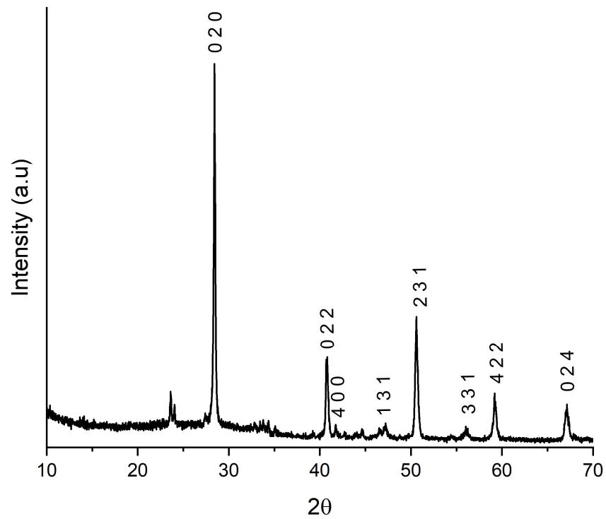
**Figure S2.** Powder XRD pattern of synthesized  $\text{BaCeO}_3$
