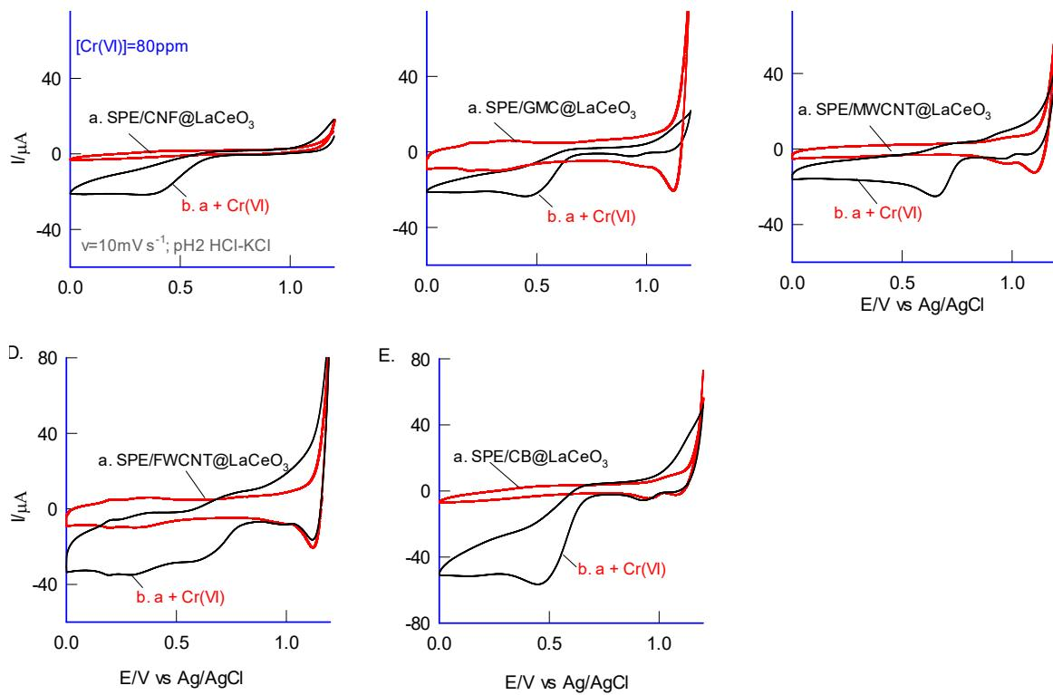
**Figure S6.** A) CV responses for catalytic reduction of Cr(VI) using different modified SPEs: A) SPE/CNF@LaCeO<sub>3</sub>; B) SPE/GMC@LaCeO<sub>3</sub>; C) SPE/MWCNT@LaCeO<sub>3</sub>; D) SPE/FWCNT@LaCeO<sub>3</sub>; E) SPE/CB@LaCeO<sub>3</sub> (Where, CB- Carbon black, CNF- Carbon nanofibers, GMC- Graphitized mesoporous carbon, MWCNT- Multi-walled carbon nanotubes, FWCNT- Functionalized multi-walled carbon nanotubes)
