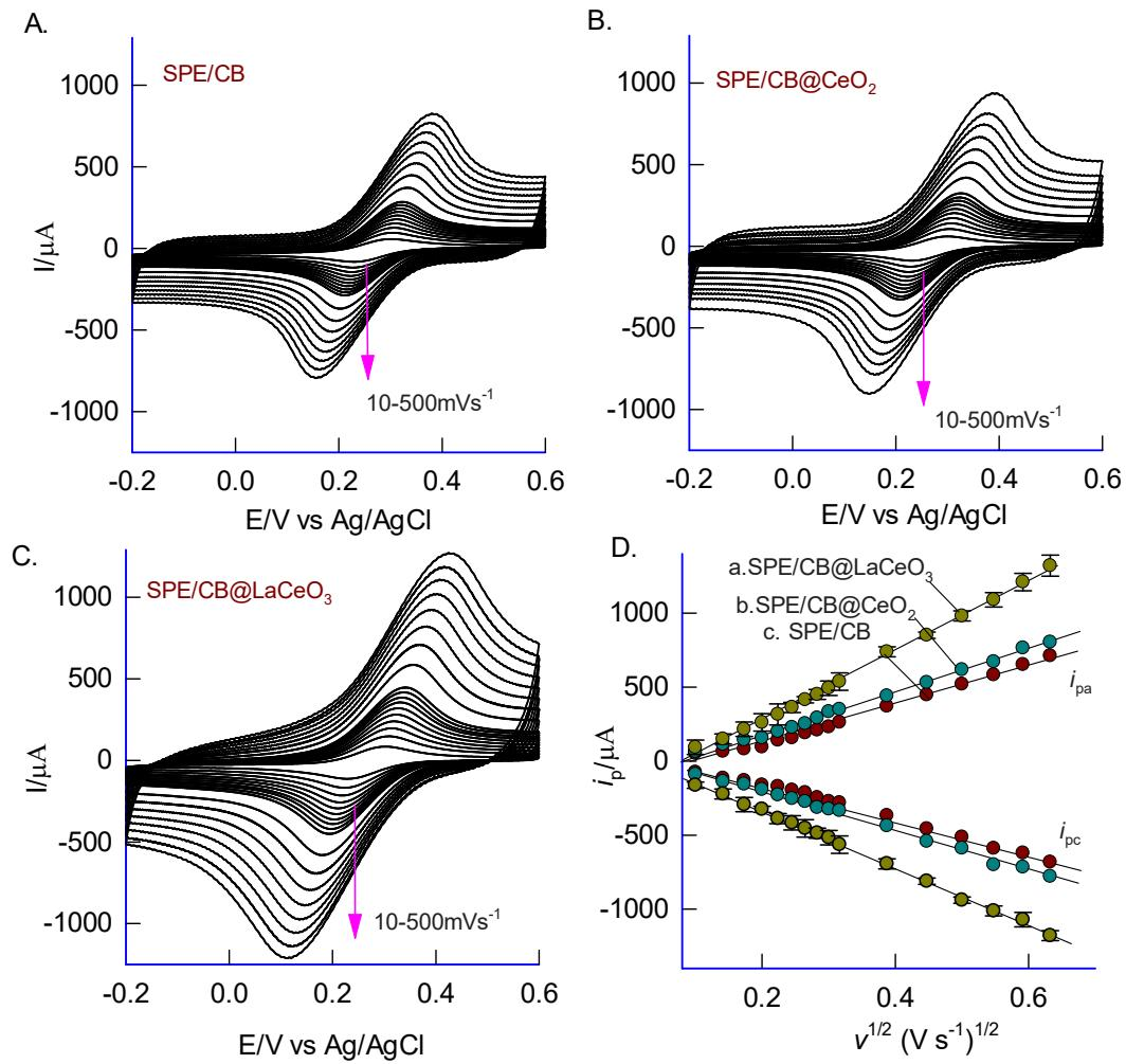
**Figure S5.** Scan rate study responses in the range 10-500 mV s<sup>-1</sup> of A) SPE/CB B) CB@CeO<sub>2</sub> and C) CB@LaCeO<sub>3</sub> in 5 mM K<sub>4</sub>[Fe(CN)<sub>6</sub>] + 0.1 M KCl at 10 mV s<sup>-1</sup> in the window -0.2 to 0.6 V vs Ag/AgCl. D)  $i_p$  vs  $v^{1/2}$  plot
