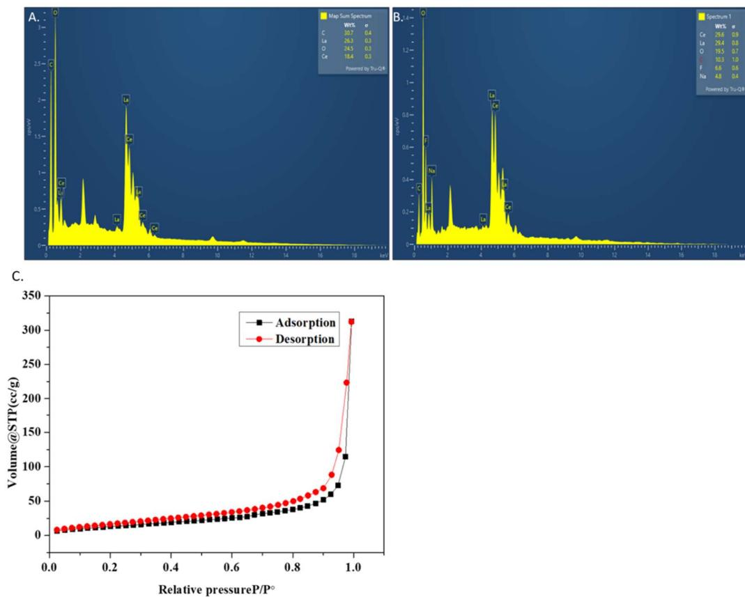
**Figure S1.** A) EDAX analysis of synthesized  $\text{LaCeO}_3$ . B) SPE modified with  $\text{CB}@\text{LaCeO}_3$  and C) BET Analysis of  $\text{LaCeO}_3$ .
