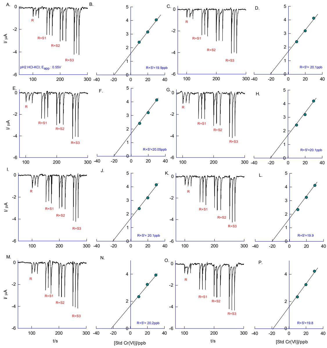
**Figure S11.** BIA method validation of Cr(VI) measurement using the developed sensor system with RO water as the sample of interest. Repeated analysis of RO water samples spiked with 20ppb Cr(VI) and followed by incremental standard additions (10, 20, 30ppb) repeated eight times for t-test validation.
