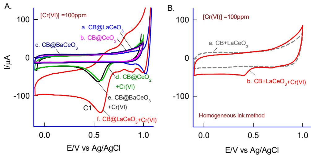
**Figure S3.** A) CV responses for catalytic reduction of Cr(VI) (curve a, b and c) using different modified SPEs along with their control experiments in absence of Cr(VI) (curve d, e and f). B) Control experiment with homogenous ink drop-casted on electrode surface to obtain SPE/CB+LaCeO<sub>3</sub> without (curve a) and with Cr(VI) (curve b).
