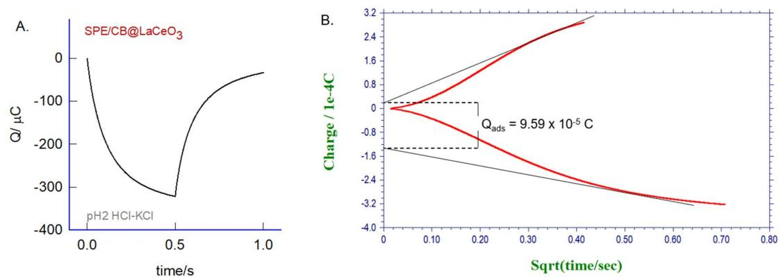
**Figure S4.** A) Chronocoulometric experiment with SPE/CB@LaCeO<sub>3</sub> in the potential window 0.8 to 0.0V vs Ag/AgCl. B) Charge *vs* root of time response corresponding to A.
