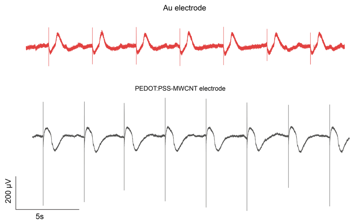
17 Figure S2. Representative field potential waveforms were recorded from cardiomyocytes cultured 18 on bare gold and PEDOT: PSS-MWCNT electrodes on day 7.
