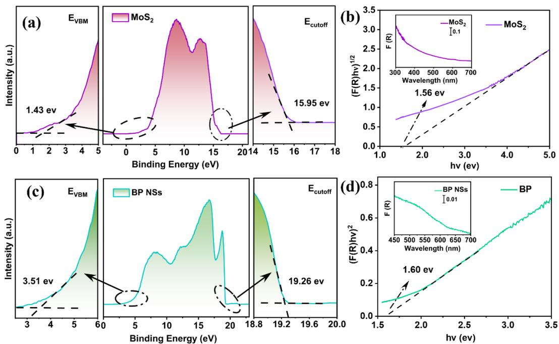
**Figure S3.** (a) UPS spectra and (b) Kubelka-Munk plots converted from the UV-vis spectra of MoS<sub>2</sub>. (c) UPS spectra and (d) Kubelka-Munk plots converted from the UV-vis spectra of BP NSs.
