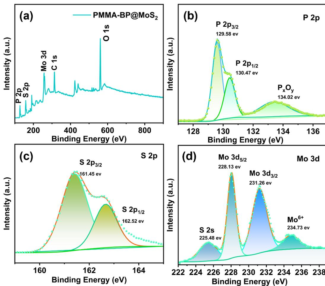
**Figure S1.** (a) XPS survey spectrum and (b-d) the corresponding high-resolution spectra of P 2p, S 2p and Mo 3d, of PMMA-BP@MoS<sub>2</sub> prepared with the concentration ratio of 1: 6.
