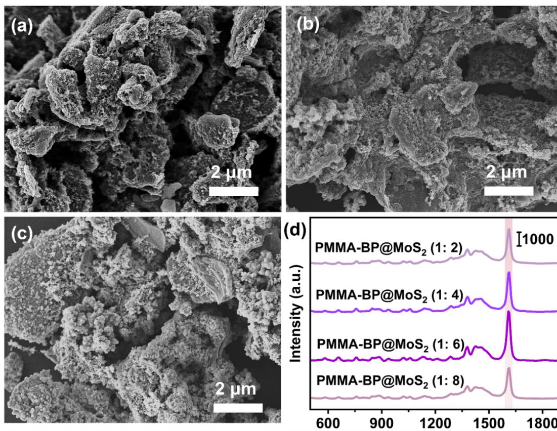
**Figure S2.** SEM images of BP@MoS<sub>2</sub> nanocomposites synthesized with different relative concentration ratios of BP and MoS<sub>2</sub>: (a) 1: 2, (b) 1: 4, and (c) 1: 8. (d) The corresponding variation of SERS strength of peak at 1621 cm<sup>-1</sup>.
