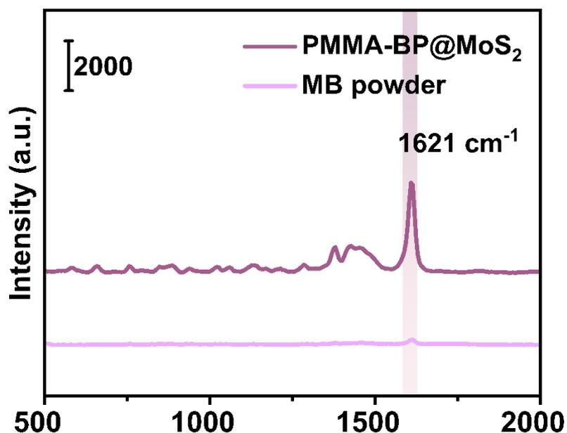
**Figure S4.** SERS spectrum of MB ( $10^{-5}$  M) from PMMA-BP@MoS<sub>2</sub> nanocomposites and Raman spectrum of MB powder.
