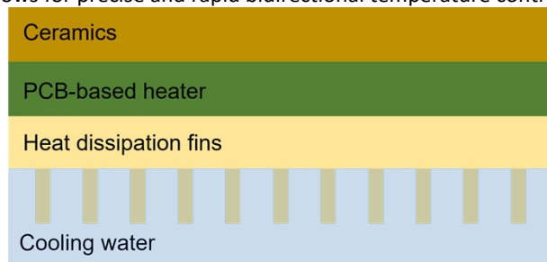
Fig. S1. Conceptual schematic of the multi-layer PCB-based heater-sensor
