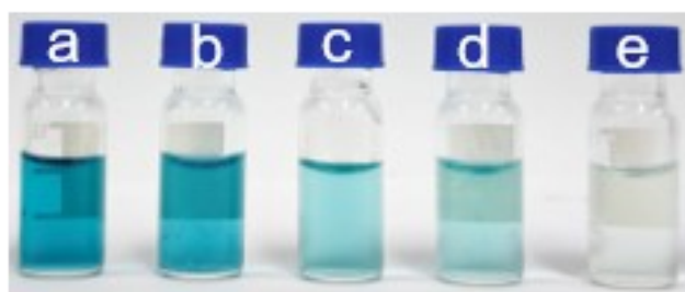
Fig. S14 The color change of CuNCs + TMB+ H 2 O 2 (a) with the scavengers of TU (b), p -BQ (c), His (d) and the mixed three scavengers (e), respectively, and the concentration of the three scavengers was all 0.1 mM.
