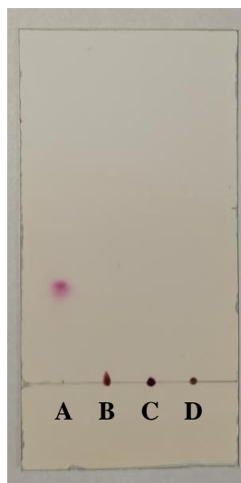
Figure S1. Thin-layer chromatographic analysis of aniline and three amino polymers with dichloromethane as the developing solvent. A: aniline, B: PEA, C: PIBA, D: Mannich.
